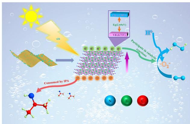
Fig. 6 Proposed photocatalytic mechanism for the Ti-C<sub>3</sub>N<sub>4</sub>-100 photocatalyst.
