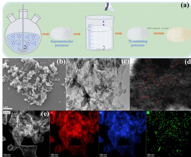
Fig. 1 (a) Schematic illustration of the preparation of  $\text{Ti-C}_3\text{N}_4$ -100. (b) The SEM, (c) TEM, and (d) HAADF-STEM images of  $\text{Ti-C}_3\text{N}_4$ -100. The (e) HAADF-STEM elemental mapping images of  $\text{Ti-C}_3\text{N}_4$ -100.
