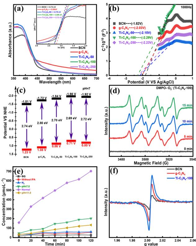
Fig. 5 (a) UV-vis diffuse reflectance spectra and band gap (higher-middle inset), (b) Mott-Schottky plots and (c) electronic band structures of all samples. (d) ESR spectrum of DMPO- $\text{O}_2^-$  in the presence of Ti-C<sub>3</sub>N<sub>4</sub>-100, (e) photocatalytic performance of Ti-C<sub>3</sub>N<sub>4</sub>-100 under different conditions, and (f) EPR spectra of BCN, g-C<sub>3</sub>N<sub>4</sub> and Ti-C<sub>3</sub>N<sub>4</sub>-100.
