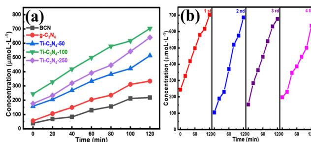
Fig. 3 (a) The photocatalytic hydrogen peroxide production performance of each sample. (b) Recycling performance of Ti-C<sub>3</sub>N<sub>4</sub>-100 photocatalyst.
