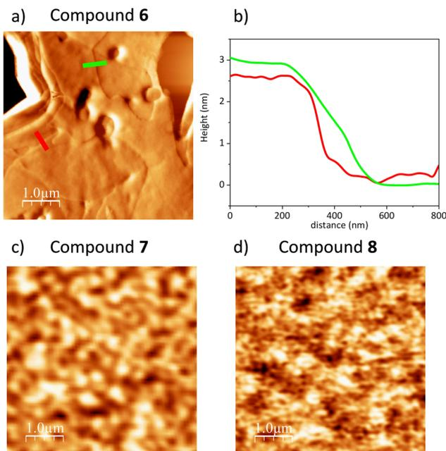
**Fig. 3** (a) AFM error signal  $5 \times 5 \mu\text{m}$  image of compound **6** OTFT device; (b) line profile acquired from topography image corresponding to Fig. 3a, reported in Fig. S3 (ESI†). The line colours correspond to the line reported in Fig. 4d; (c) and (d) AFM topography  $5 \times 5 \mu\text{m}$  image of compound **7** and **8** top surface OTFT device, respectively.
