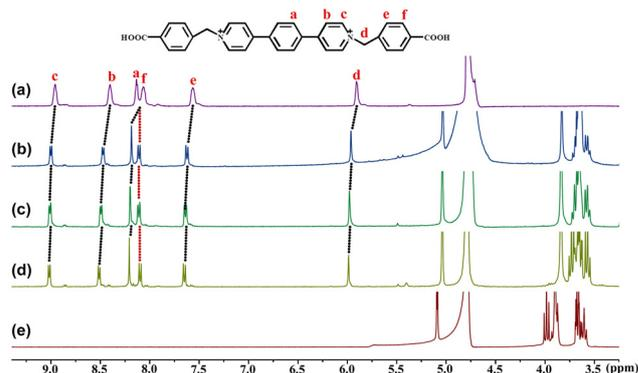
Fig. 2 <sup>1</sup>H NMR spectra (400 MHz, D<sub>2</sub>O) of the 3<sup>2+</sup> (4.0 mmol L<sup>-1</sup>, a) binding with (b) 0.52, (c) 1.13, and (d) 2.11 equiv. of  $\beta$ -CD in D<sub>2</sub>O at 20 °C. (e) The <sup>1</sup>H NMR spectrum (400 MHz, D<sub>2</sub>O) of  $\beta$ -CD in D<sub>2</sub>O (5.0 mmol L<sup>-1</sup>) at 20 °C.
