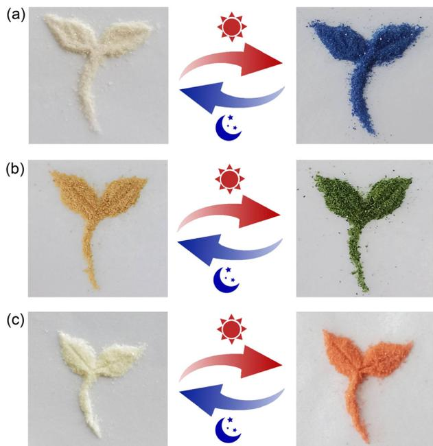
Fig. 3 Photographs showing the photochromic performances of the inclusion complexes  $1^{2+}@β\text{-CD}$  (a),  $2^{2+}@β\text{-CD}_2$  (b) and  $3^{2+}@β\text{-CD}_2$  (c) upon light irradiation with a xenon lamp.
