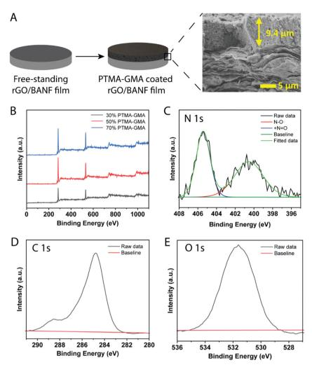
Fig. 1 (A) Schematic representation of structural cathode preparation. (B) XPS Survey scans for 30 wt%, 50 wt%, 70 wt% PTMA-GMA on rGO/BANF. High-resolution XPS spectra for 50 wt% PTMA-GMA on rGO/BANF (C) N 1s peak with deconvolution, (D) C 1s peak, and (E) O 1s peak.
