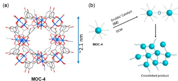
Fig. 6 (a) Synchrotron single crystal X-ray structure of **MOC-4** displaying the core **MOC** as the disordered alkyl chains could not be resolved crystallographically. (b) Cartoon depicting the cross-linking process *via* G2 Grubbs' catalyst in DCM. Reproduced from ref. 52 with permission from ACS, copyright 2019.
