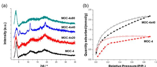
Fig. 7 (a) Powder XRD patterns of the **MOC-4** and the supramolecular cross-linked products. (b)  $\text{CO}_2$  adsorption experiments carried out at 195 K and 1.2 bar. Reproduced from ref. 52 with permission from ACS, copyright 2019.
