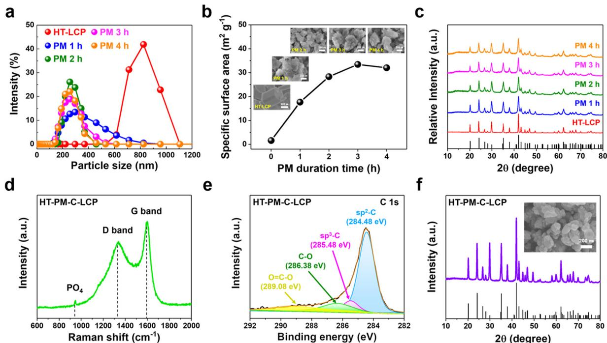
Fig. 2 Characterization of HT-LCP crystals after post-synthesis modifications (high-energy PM and conductive C-coating) *via* (a) size-distribution measurement with the dynamic light scattering, (b) BET analysis, and (c) XRD with different milling duration time; (d) Raman, (e) XPS C 1s spectra, and (f) XRD.
