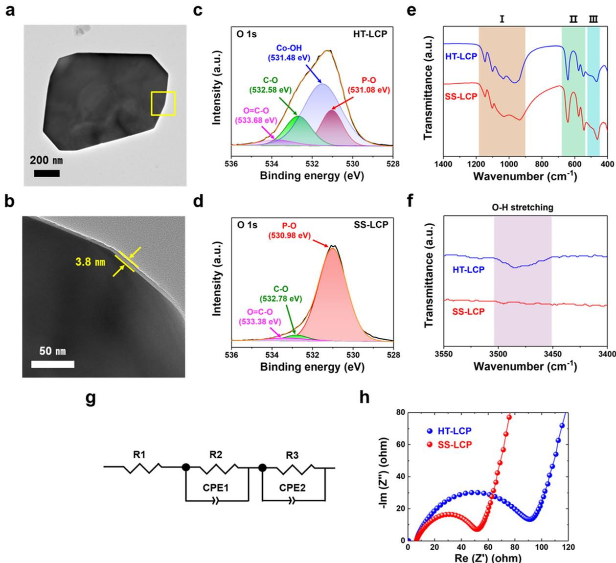
Fig. 4 Characterization of nano-scale  $\text{Co}(\text{OH})_2$  layer on the surface of HT-LCP. (a) and (b) TEM and HRTEM images of HT-LCP; (c) and (d) XPS O 1s and (e) and (f) FTIR spectra of HT-LCP and SS-LCP; (g) and (h) Nyquist plots of pristine HT-LCP and SS-LCP electrodes with equivalent circuit used to fit the EIS model.
