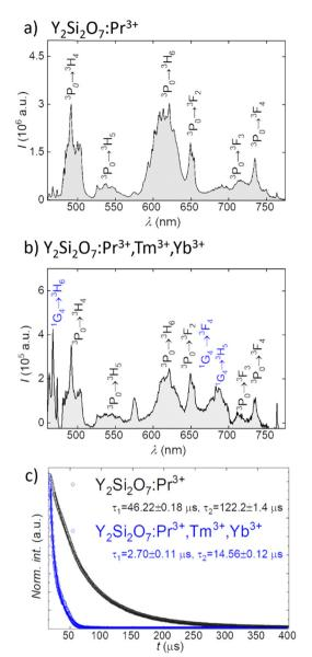
**Fig. 2** Down-conversion emission spectra of  $Y_2Si_2O_7$ : $Pr^{3+}$  (a) and  $Y_2Si_2O_7$ : $Pr^{3+}$ , $Trm^{3+}$ , $Yb^{3+}$  (b) phosphors upon 447 nm excitation together with fluorescence decay curves recorded at 610 nm upon 447 nm excitation for  $Pr^{3+}$ -based  $Y_2Si_2O_7$  silicates (c).
