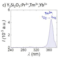
**Fig. 3** Vis-to-UVC UC spectra of  $Y_2Si_2O_7:Pr^{3+}$  (a) and  $Y_2Si_2O_7:Pr^{3+}$ , $T-m^{3+}$ , $Yb^{3+}$  (b) powders upon 447 nm CW laser irradiation at a power of 1000 mW. The insets show log-log plots of integrated intensity vs excitation power with the linear fits and slope values. NIR-to-UV UC spectrum of  $Y_2Si_2O_7:Pr^{3+}$ , $Tm^{3+}$ , $Yb^{3+}$  (c) upon 980 nm CW laser irradiation at a power of 1000 mW.
