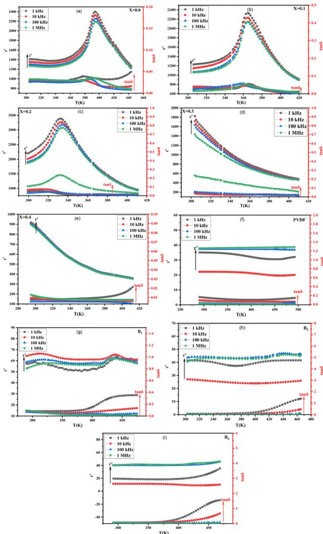
Fig. 9 (a)–(i)  $\epsilon'$  and  $\tan \delta$  vs. temperature at different frequencies of  $\text{Ba}_{1-x}\text{Sr}_x\text{TiO}_3$  (where  $x = 0.0, 0.1, 0.2, 0.3,$  and  $0.4$ ) samples, pure PVDF, and  $B_1, B_2,$  and  $B_3$  composites.
