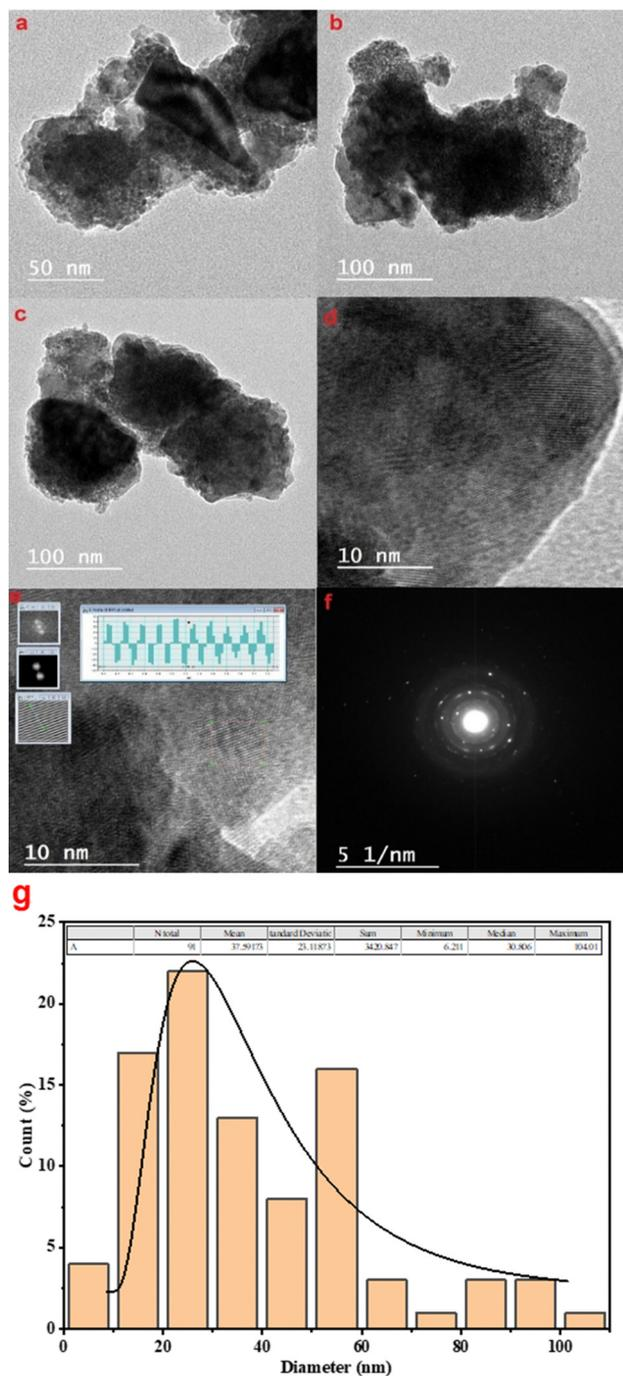
Fig. 7 (a)–(c) TEM micrographs of BaTiO<sub>3</sub> in the diffraction mode, (d) and (e) HRTEM images, (f) selected area electron diffraction (SAED) pattern, and (g) particle size distribution histogram.
