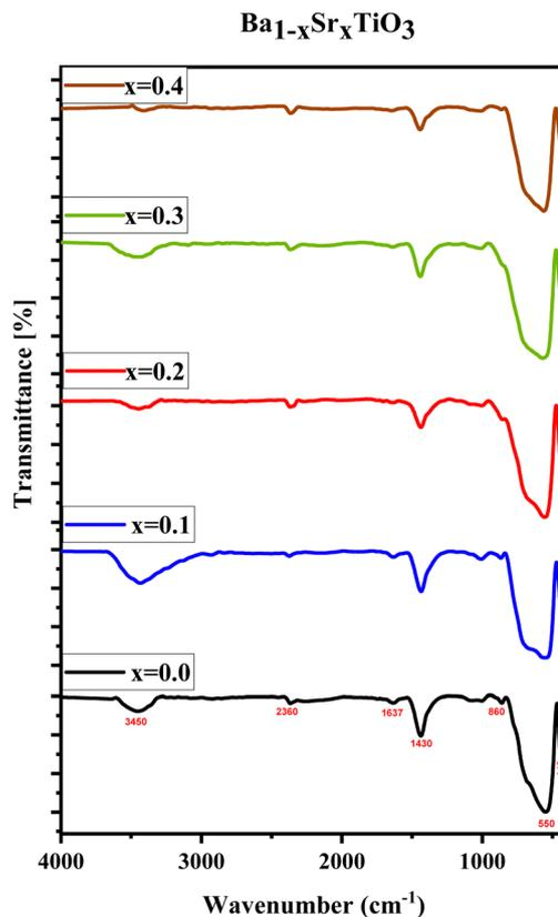
Fig. 4 FTIR spectra of  $Ba_{1-x}Sr_xTiO_3$  (where  $x = 0.0, 0.1, 0.2, 0.3$ , and  $0.4$ ).
