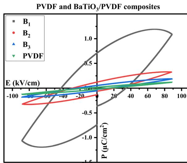
**Fig. 12** *P*-*E* hysteresis loops samples, pure PVDF, B<sub>1</sub>, B<sub>2</sub>, and B<sub>3</sub> composites.
