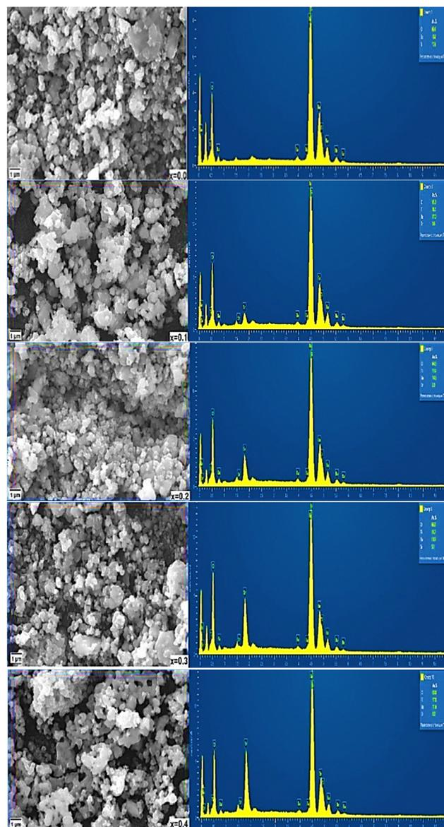
Fig. 8 SEM micrographs (left) and corresponding EDX micrographs (right) of Ba<sub>1-x</sub>Sr<sub>x</sub>TiO<sub>3</sub> (where  $x = 0.0, 0.1, 0.2, 0.3,$  and  $0.4$ ).
