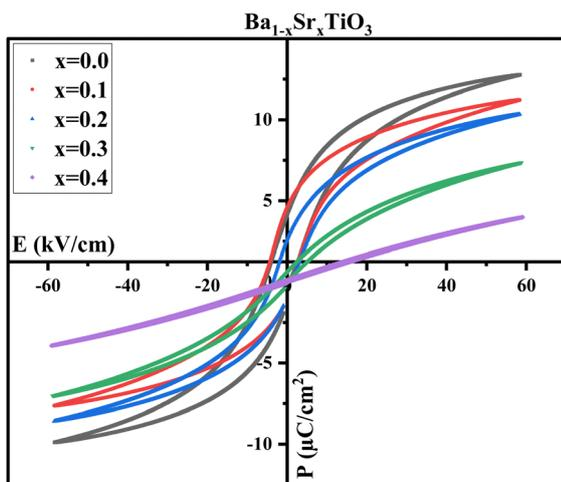
**Fig. 11** *P*-*E* hysteresis loops of Ba<sub>1-x</sub>Sr<sub>x</sub>TiO<sub>3</sub> (where *x* = 0.0, 0.1, 0.2, 0.3, and 0.4).
