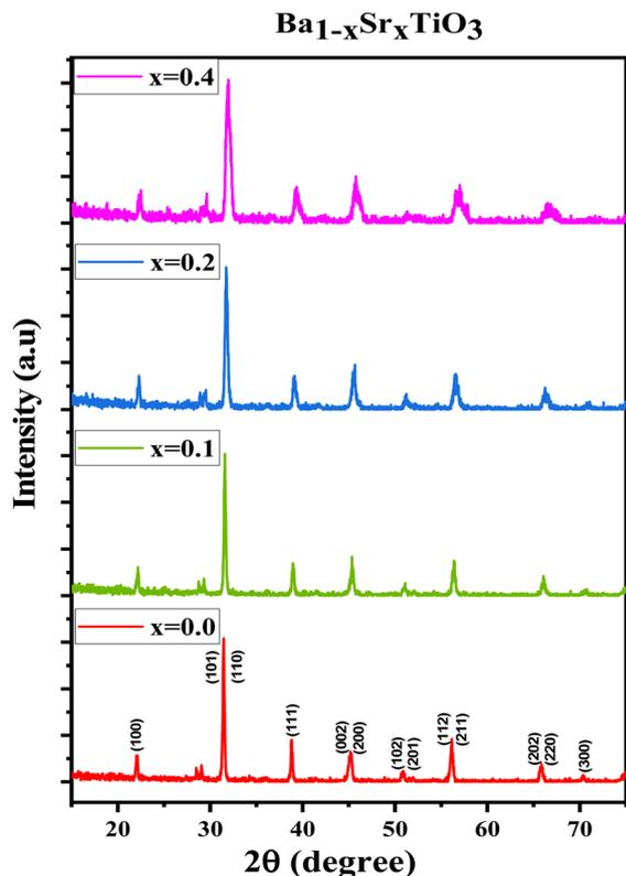
Fig. 1 XRD patterns of  $\text{Ba}_{1-x}\text{Sr}_x\text{TiO}_3$  (where  $x = 0.0, 0.1, 0.2, 0.3,$  and  $0.4$ ).
