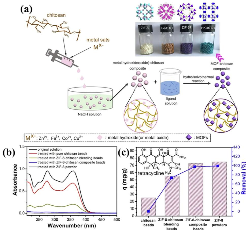
Fig. 9 (a) Diagrammatic representation of the CS/MOFs composite fabrication using the *in situ* growth method. (b) UV-vis spectra of tetracycline solution treated with different adsorbents. (c) Adsorption capability of the different adsorbents. Reproduced with permission.<sup>105</sup> Copyright 2020, Elsevier.
