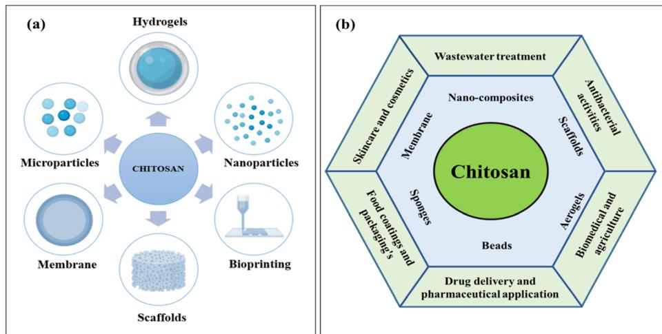
Fig. 3 (a) Different formulations of CS into hydrogels, nano-particles, membranes, scaffolds, and bio-printing, and (b) applications of CS-based materials in the field of environment, medicals and food packaging.
