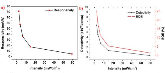
Fig. 7 Variation of (a) responsivity and (b) detectivity and EQE with the intensity of simulated solar light for the optimized sample of Mg: Pb-5:5.
