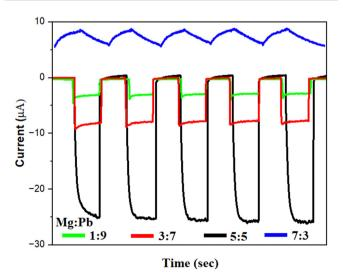
Fig. 5 Photodynamic response of devices fabricated with variation Mg: Pb stoichiometry for samples of Mg: Pb-1:9, Mg: Pb-3:7, Mg: Pb-5:5 and Mg: Pb-7:3.
