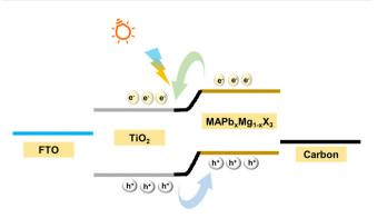
Fig. 9 Schematic illustration of the photocarrier transport in the device using the band diagram.
