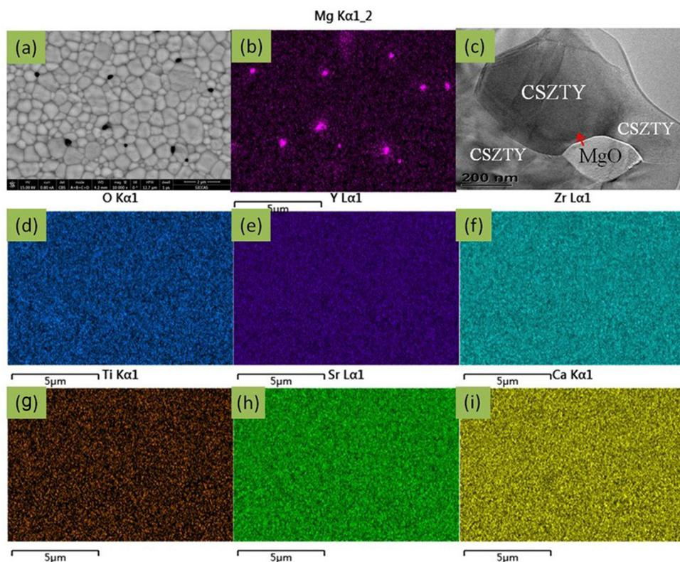
Fig. 3 (a) Cross-sectional SEM-BSE image of the CSZTY ( $x = 0.1$ ) ceramic at 10 000x magnification. The sample was surface polished and heat treated at  $1400 \text{ }^\circ\text{C}$  for 1 h. (b) and (d)–(i). The corresponding EDS elemental mapping images of Mg, O, Y, Zr, Ti, Sr, and Ca. (c) TEM-BSE image of the CSZTY ( $x = 0.1$ ) ceramic in the MgO and CSZTY grain coexisting region.
