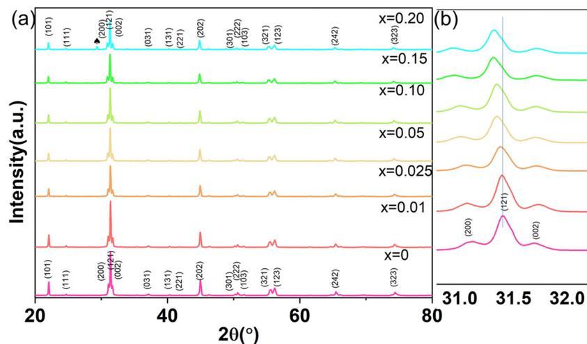
Fig. 1 (a) The XRD patterns of CSZT and CSZTY ( $x = 0.01, 0.05, 0.10, 0.15,$  and  $0.20$ ) ceramics. At  $x = 0.20$ , the XRD pattern shows a small amount of  $Y_2O_3$  which is marked with a black heart symbol. (b) Partial enlarged drawing of the XRD patterns in the  $2\theta$  range from  $31.0^\circ$  to  $32.0^\circ$ .
