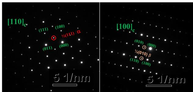
Fig. 7 SAED patterns viewed along the  $[110]_c$  and  $[100]_c$  zone axis for the CSZTY ( $x = 0.1$ ) ceramic.  $\alpha$  and  $\beta$  superlattice reflections from antiphase tilting and antiparallel shifts of A-site species are observed in  $[110]_c$  and  $[100]_c$  zone axis diffraction patterns, respectively.
