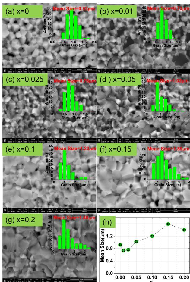
Fig. 2 (a)–(g) Cross-sectional SEM-BSE images at 10000x magnification of CSZT and CSZTY ( $x = 0.01, 0.025, 0.05, 0.10, 0.15,$  and  $0.20$ ) ceramics. The insets are the corresponding grain size distribution diagram. (h) Diagram of the mean grain sizes of CSZTY ceramics with different  $x$ .
