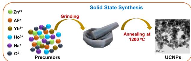
Scheme 1 Schematic illustration demonstrating the synthesis of  $\text{ZnAl}_2\text{O}_4$ : 1% $\text{Ho}^{3+}$ , 5% $\text{Yb}^{3+}$ ,  $x\%\text{Na}^+$  ( $x = 0, 1, 2, 5, 7,$  and  $10$  mol%) UCNPs.
