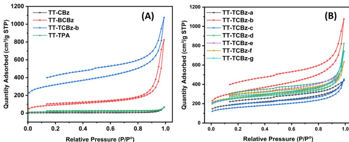
Fig. 4 (A) Stacked  $N_2$  adsorption–desorption isotherms of TT-CBz, TT-BCBz, TT-TCBz-b and TT-TPA. (B) Stacked  $N_2$  adsorption–desorption isotherms of TT-TCBz-a, TT-TCBz-b, TT-TCBz-c, TT-TCBz-d, TT-TCBz-e, TT-TCBz-f, and TT-TCBz-g, respectively.
