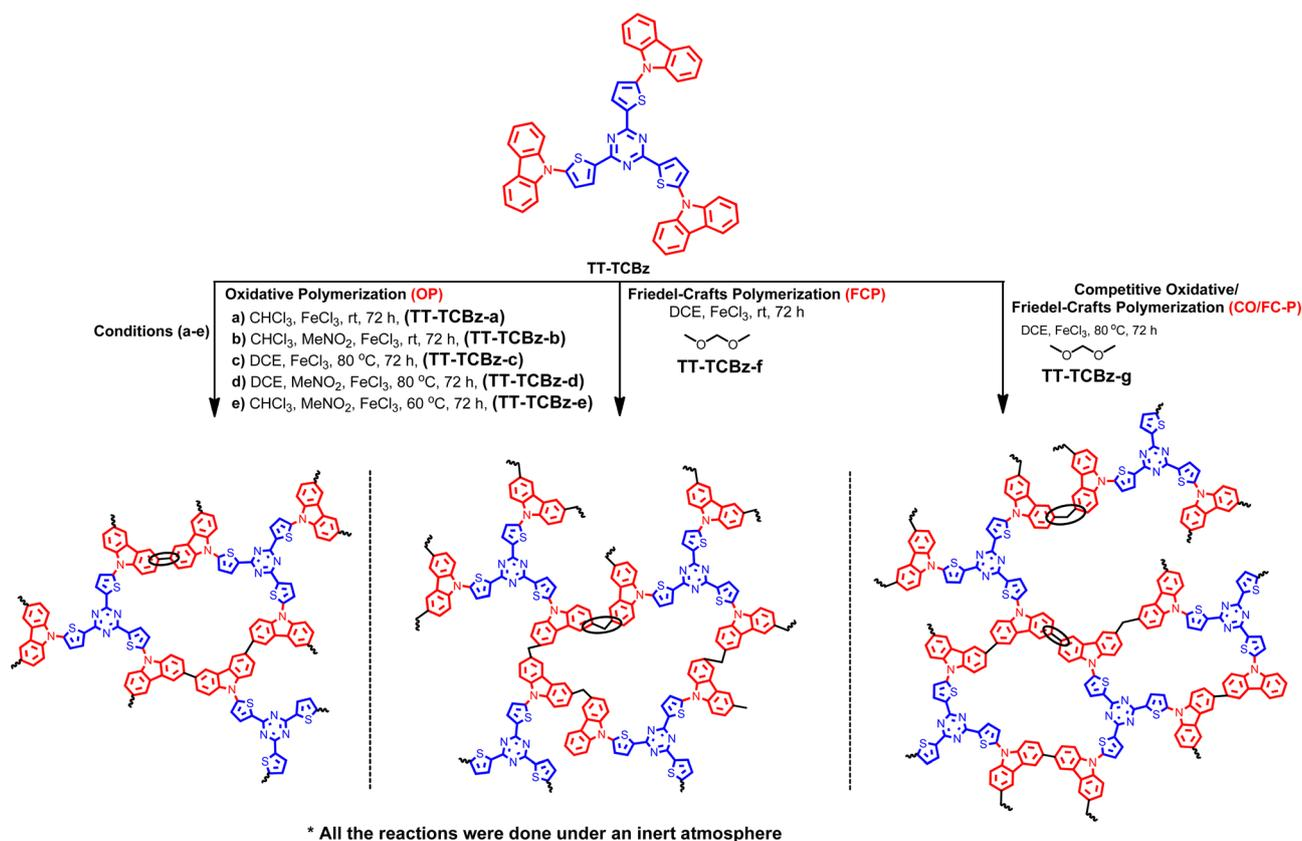
Scheme 2 Polymerization of **TT-TCBz** under different reaction conditions in the presence of FeCl<sub>3</sub> to give polymers **TT-TCBz-a**, **TT-TCBz-b**, **TT-TCBz-c**, **TT-TCBz-d**, **TT-TCBz-e**, **TT-TCBz-f**, and **TT-TCBz-g**, respectively.
