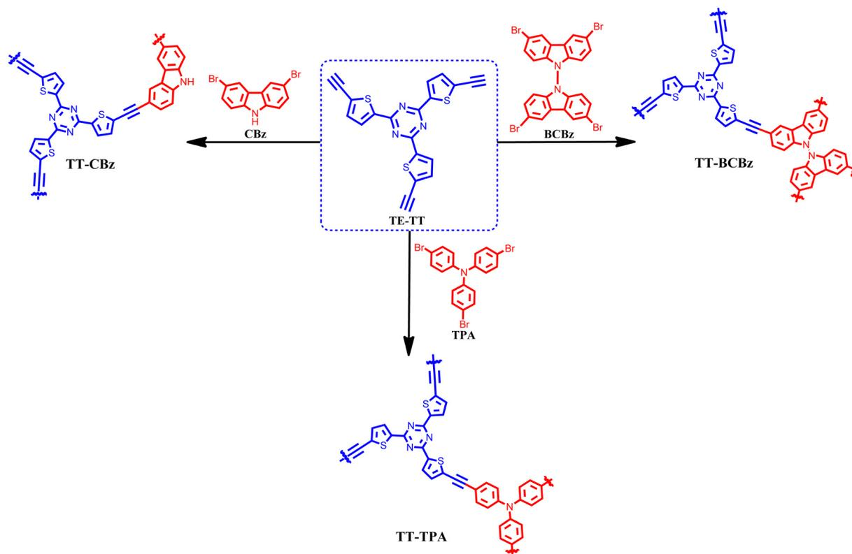
Scheme 1 Synthesis of thienyltriazine-based CPPs **TT-CBz**, **TT-BCBz** and **TT-TPA**.
