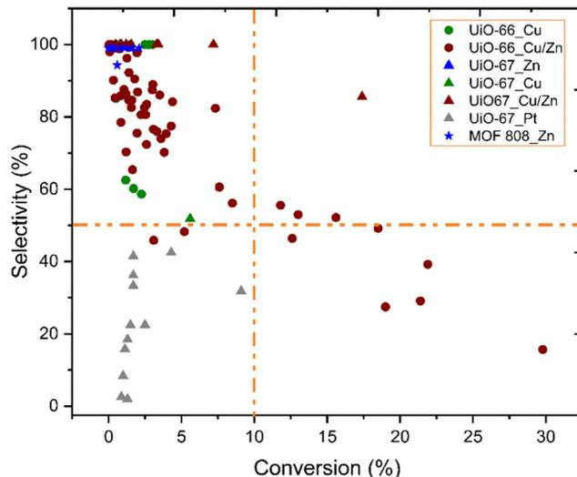
Fig. 10 Selectivity toward methanol versus conversion of CO<sub>2</sub>. While different symbols represent various metal-organic frameworks, different colours represent various incorporated metal active sites.<sup>37–46</sup> Orange dashed lines represent 10% conversion and 50% selectivity and have been included to guide the eyes.
