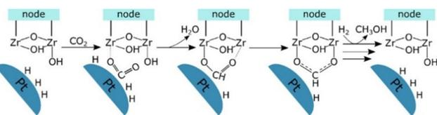
Fig. 15 Schematic presentation of the postulated reaction mechanism of CO<sub>2</sub> hydrogenation to the formate intermediate in CH<sub>3</sub>OH formation at the Pt–Zr node interface. Reprinted with permission from ref. 45. Copyright 2020 American Chemical Society (<https://pubs.acs.org/doi/10.1021/jacs.9b10873>).
