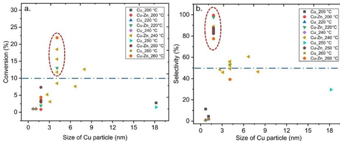
Fig. 13 (a) Conversion of  $\text{CO}_2$  versus size of Cu particle. (b) Selectivity towards methanol versus size of Cu particle. Blue dashed lines represent 10% conversion and 50% selectivity.
