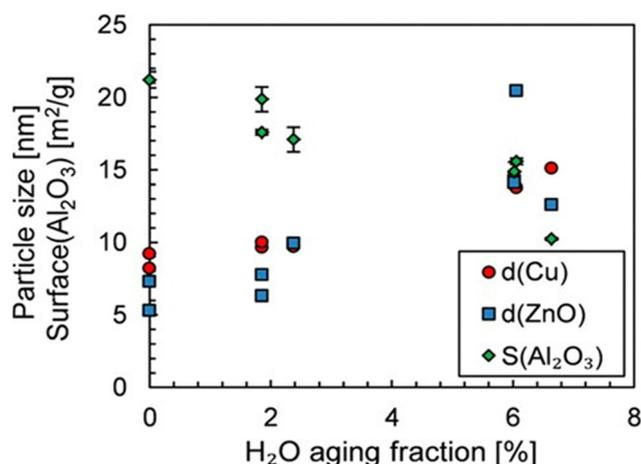
Fig. 6 Influence of H<sub>2</sub>O volume fraction on the Cu and ZnO particle size and Al<sub>2</sub>O<sub>3</sub> surface. The aging period was 48 hours. Reprinted with permission from ref. 85. Copyright 2019 American Chemical Society (<https://pubs.acs.org/doi/full/10.1021/acs.iecr.9b01898>).
