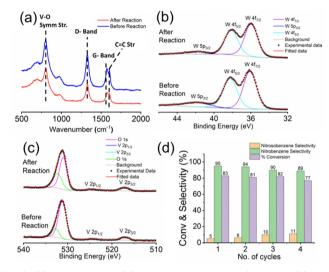
Fig. 6 (a) Raman spectra, (b) high-resolution W 4f XPS scan and (c) highresolution V 2p XPS scan of the micro-catalytic reactor trail recorded before and after performing the reaction. (d) Reusability of the microcatalytic trails: % conversion and product selectivity towards nitrobenzene and nitrosobenzene over four cycles following the reaction conditions mentioned in Table 1, entry 5.
