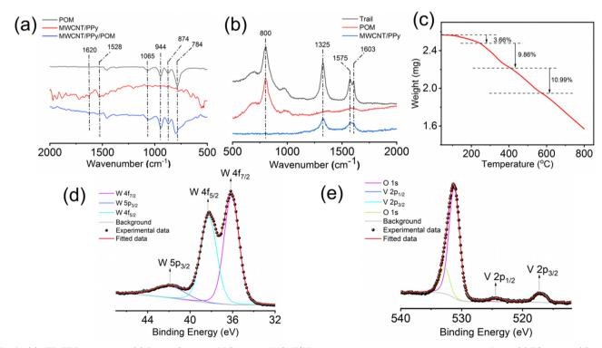
Fig. 4 (a) ATR-FTIR spectra and (b) Raman Spectra of POM, the MWCNT/PPy composite and the optically patterned trail, and (c) TGA curve, (d) highresolution W 4f X-ray photoelectron spectra and (e) high-resolution V 2p X-ray photoelectron spectra of the MWCNT/PPy/POM composite (obtained by scrapping off materials from the fabricated trails).
