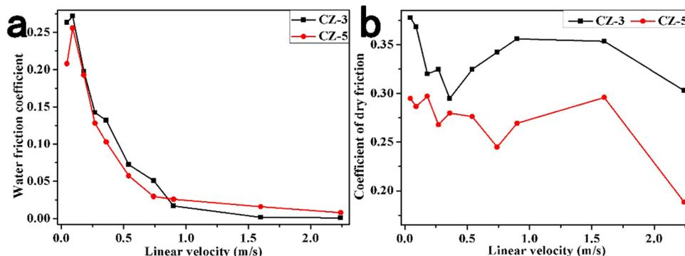
Fig. 6 The tribological properties of the PEK-C/graphite composites: (a) water friction coefficient; (b) coefficient of dry friction.
