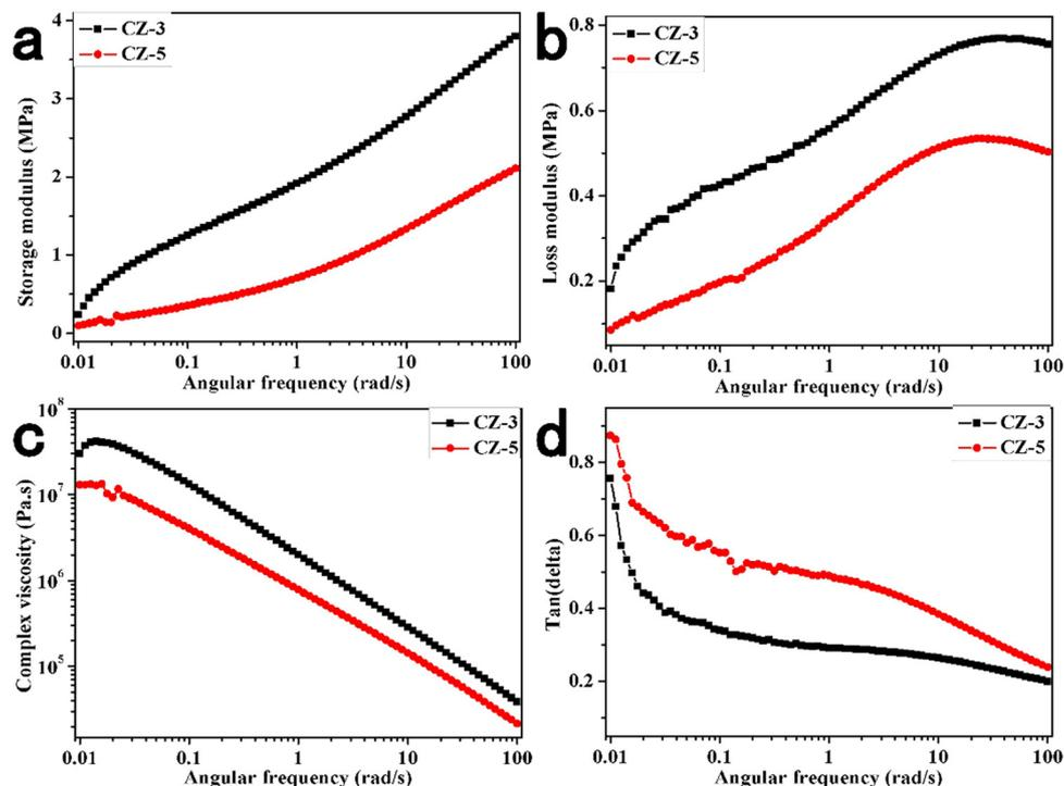
Fig. 4 The melt rheological properties of the PEK-C/graphite composites: (a)–(d) the evolution of the storage modulus ( $G'$ ), loss modulus ( $G''$ ), complex viscosity ( $|\eta^*|$ ) and loss angle tangent ( $\tan \delta$ ) versus angular frequency at 320 °C, respectively.
