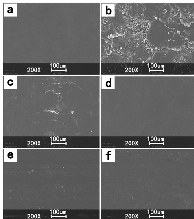
Fig. 7 SEM micrographs of worn surfaces of the PEK-C/graphite composites: (a) the surface of CZ-3 before friction testing; (b) the friction surface of CZ-3 after dry sliding; (c) the friction surface of CZ-3 after water lubrication; (d) the surface of CZ-5 before friction testing; (e) the friction surface of CZ-5 after dry sliding; (f) the friction surface of CZ-5 after water lubrication.
