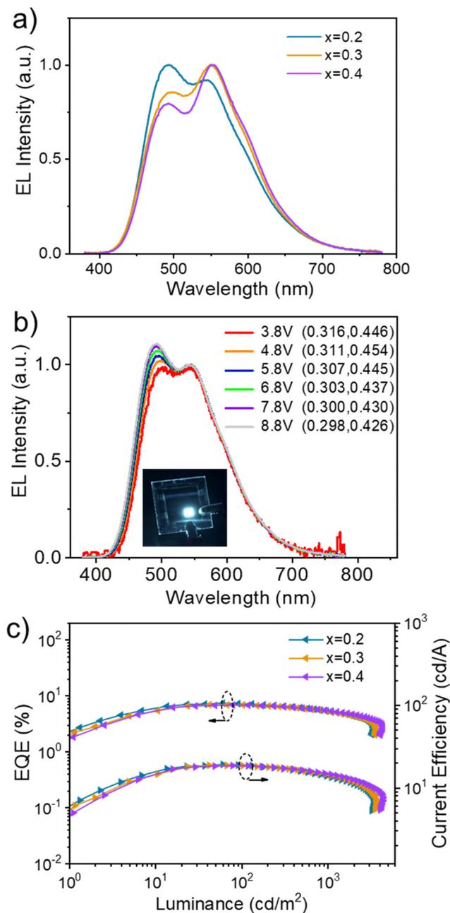
**Fig. 4** Device performance of solution-processed white OLEDs with 0.2–0.4 wt% TBRb: (a) EL spectra recorded at 1000 cd m<sup>-2</sup>. (b) Driving voltage dependence on EL spectra for 0.2 wt% TBRb. Inset: Plot of the corresponding white light device. (c) EQE and current efficiency as a function of luminance.
