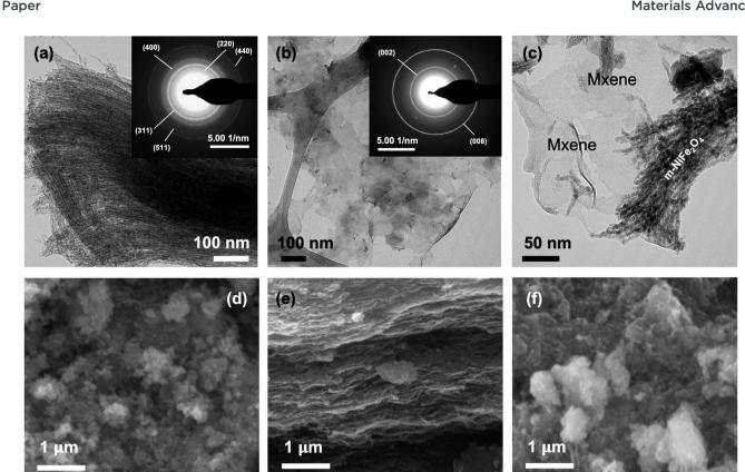
Fig. 2 (a-c) TEM images (insets: SAED analyses) and (d-f) SEM images of m-NiFe<sub>2</sub>O<sub>4</sub>, MXene, and m-NiFe<sub>2</sub>O<sub>4</sub>/Mxene composite, respectively.
