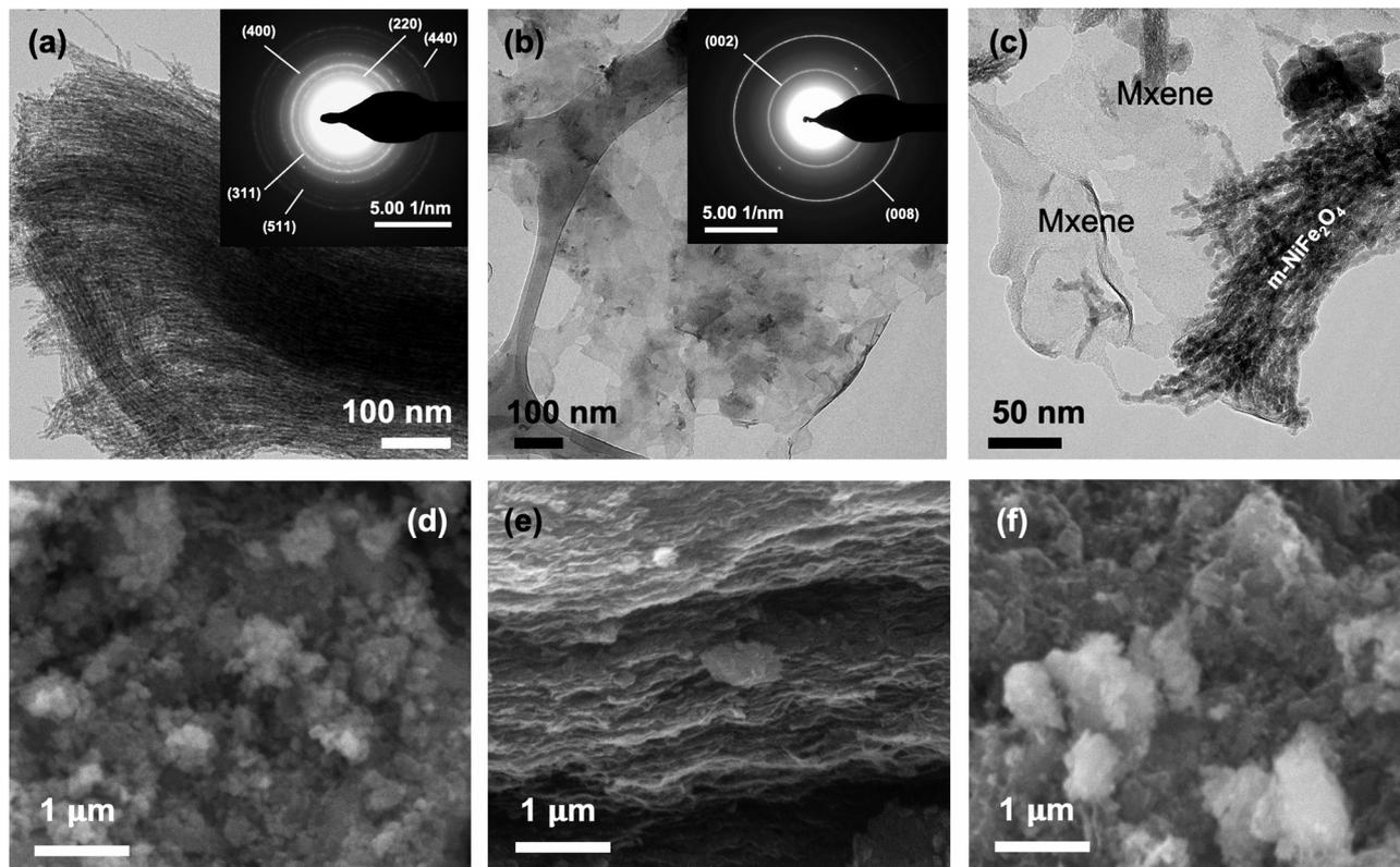
Fig. 2 (a–c) TEM images (insets: SAED analyses) and (d–f) SEM images of *m*-NiFe<sub>2</sub>O<sub>4</sub>, MXene, and *m*-NiFe<sub>2</sub>O<sub>4</sub>/MXene composite, respectively.
