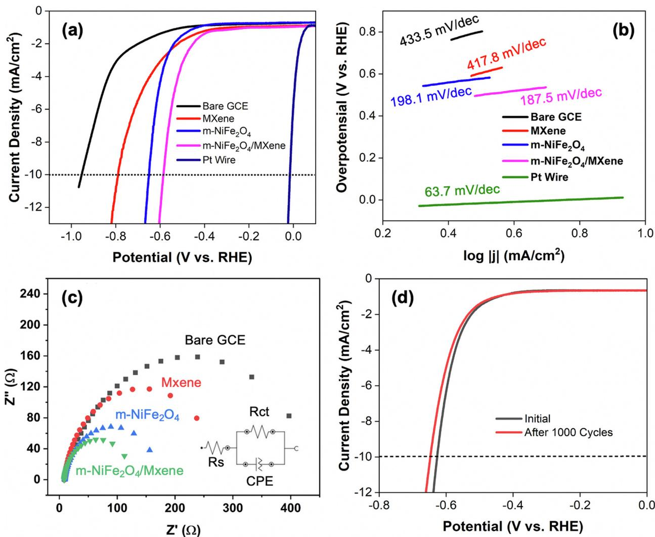
Fig. 3 (a) Polarization curves of bare GCE, MXene,  $m$ -NiFe<sub>2</sub>O<sub>4</sub>,  $m$ -NiFe<sub>2</sub>O<sub>4</sub>/MXene, and Pt Wire at 1M NaOH, (b) the corresponding Tafel plots, (c) and Nyquist plots obtained from the electrochemical impedance spectroscopy (EIS) analysis and (d) polarization curves of  $m$ -NiFe<sub>2</sub>O<sub>4</sub>/MXene before and after 1000 cycles.
