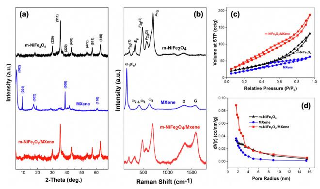
Fig. 1 (a) XRD patterns, (b) Raman spectra, (c)  $N_2$  adsorption–desorption isotherms, and (d) pore size distribution plots of m-NiFe<sub>2</sub>O<sub>4</sub>, MXene, and m-NiFe<sub>2</sub>O<sub>4</sub>/Mxene composite.
