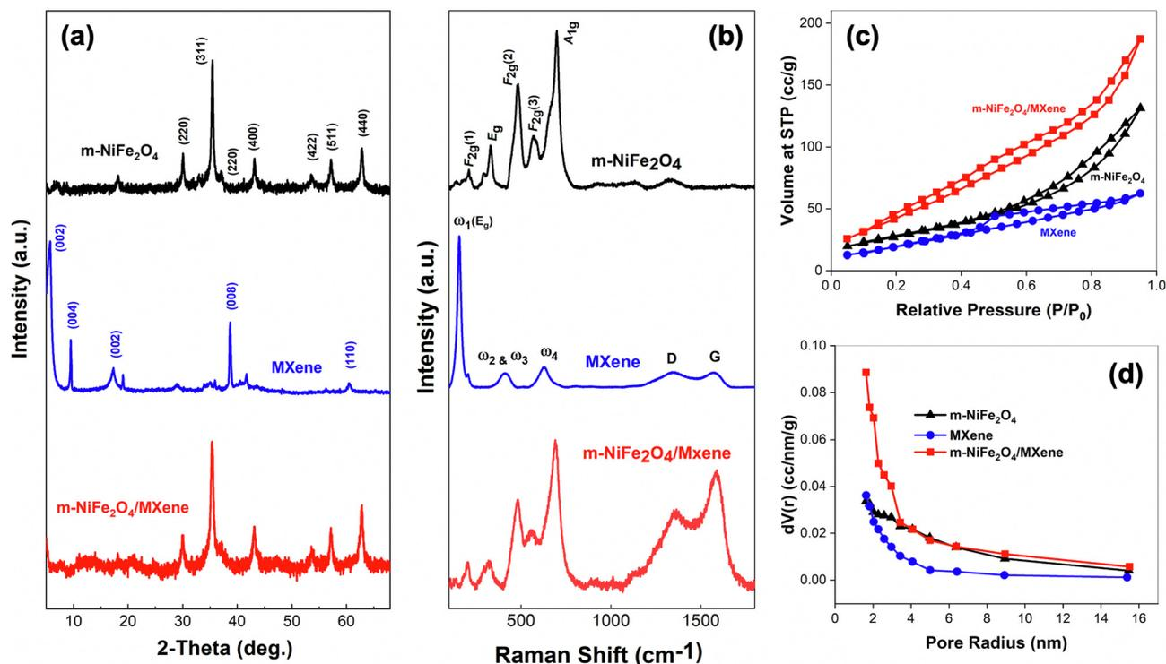
Fig. 1 (a) XRD patterns, (b) Raman spectra, (c)  $\text{N}_2$  adsorption–desorption isotherms, and (d) pore size distribution plots of  $m\text{-NiFe}_2\text{O}_4$ , MXene, and  $m\text{-NiFe}_2\text{O}_4/\text{MXene}$  composite.
