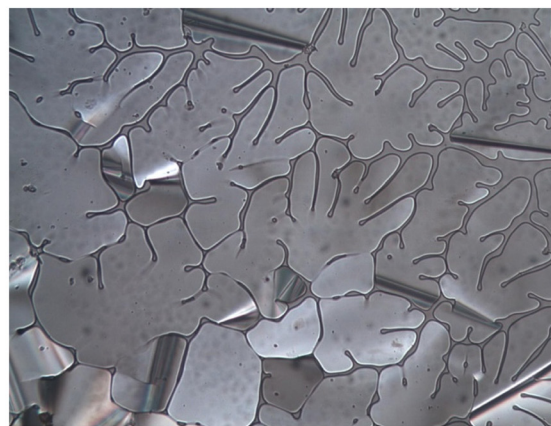
Fig. 2 (Left) DSC curves for Series I compounds. (Right) Compound 2 at 229 °C while cooling from isotropic liquid viewed through crossed polarizers.
