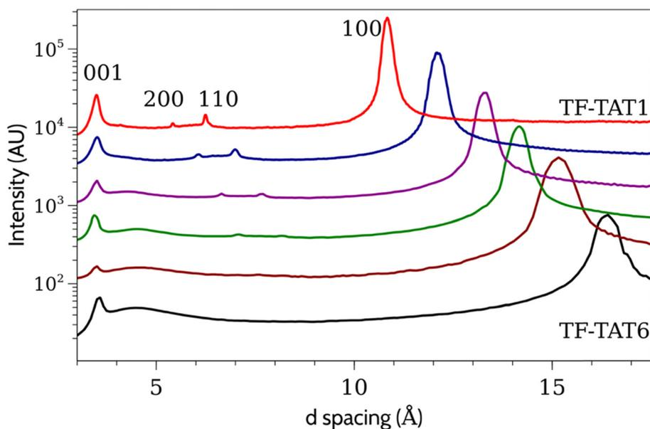
**Fig. 4** SAXS patterns for compounds 1–6 showing the evolution of the mesophase structure as the tail lengths are changed. The intercolumn distance ranges from approximately 17 Å down to 11 Å, which is approximately the diameter of the molecules. The broad diffuse scattering near 4 Å comes from the tails and can be seen to diminish until it is almost completely absent for TF-TAT1.
