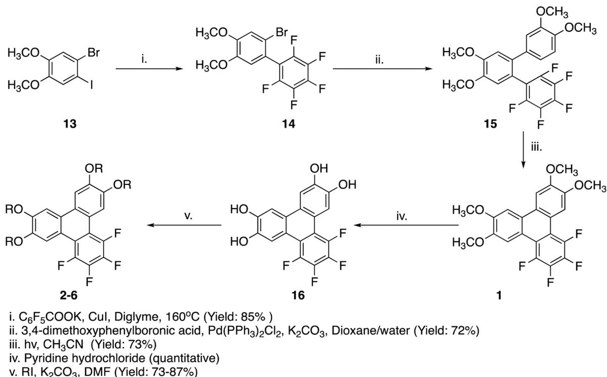
Scheme 1 Synthesis of Series I (TF-TAT $n$ ) 1,2,3,4-tetrafluoro-6,7,10,11-tetraalkoxytriphenylenes.
