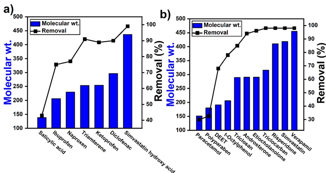
Fig. 8 Correlation of molecular weight of (a) negatively charged, and (b) neutral pharmaceuticals and personal care product vs. cellulose acetate membrane.<sup>303</sup>
