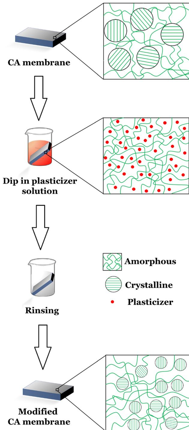
Fig. 5 Schematic illustration of a proposed mechanism for the role of plasticizer on the crystalline structure of the cellulose acetate (CA) membrane.<sup>254</sup> The pristine CA membrane consists large crystallites embedded in amorphous regions. Soaking of the membrane in plasticizer solutions leads to the swelling of both the crystalline and amorphous regions. Plasticizer is gradually released by water rinsing, resulting in the rearrangement and recrystallization of the polymer chains.
