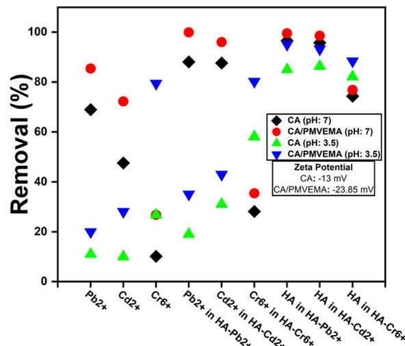
Fig. 10 Influence of pH, polymer composition, and addition of negatively-charged organic compound on removal rate of three heavy metals ( $\text{Pb}^{2+}$ ,  $\text{Cd}^{2+}$ , and  $\text{Cr}^{6+}$ ).<sup>251</sup> (Metal ion concentration = 10 ppm, Humic acid = 20 ppm, pressure = 4 bar, contact time = 2 h, rotation speed = 300 rpm, and Temperature = 25 °C).
