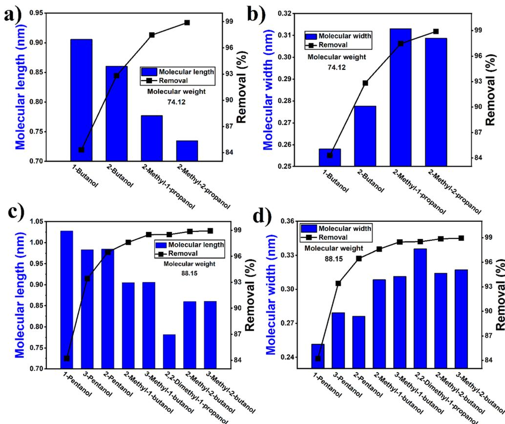
Fig. 9 Correlation of molecular size parameter of (a) and (c) molecular length, and (b) and (d) molecular width of organic pollutant vs. removal rate (%) of reverse osmosis membrane.<sup>308</sup>
