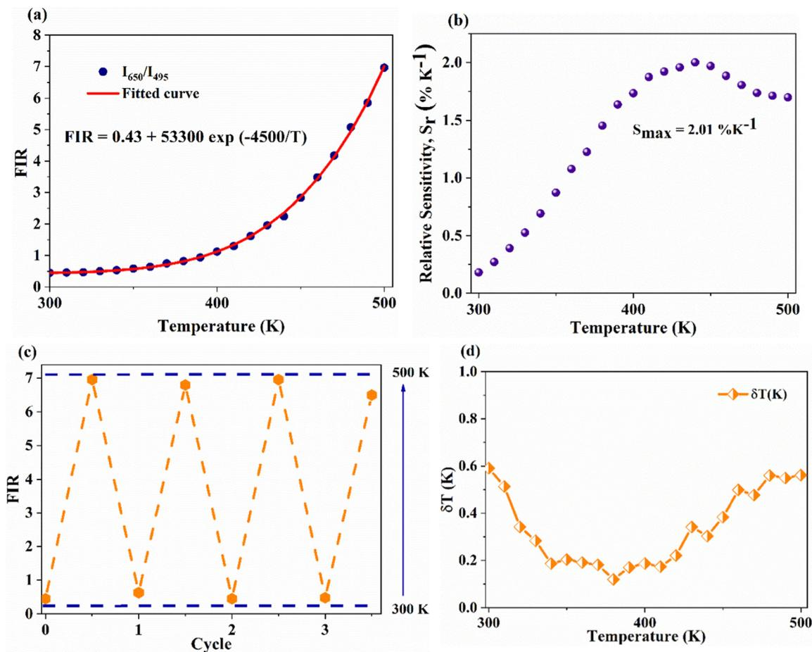
Fig. 7 (a) and (b) Variation of  $\text{FIR} \frac{I_{650}}{I_{495}}$  and relative sensitivity,  $S_r$ , with temperature, (c) temperature cycling of FIR, and (d) the temperature resolution in the temperature range 300–500 K.
