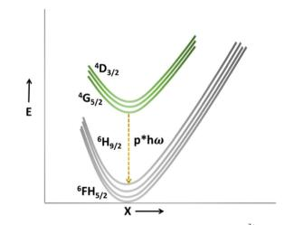
Fig. 9 Schematic model showing thermal quenching of Sm<sup>3+</sup>.
