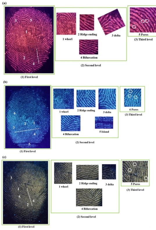
Fig. 11 Magnified features of (a) SNMV:Eu<sup>3+</sup>, (b) SNMV and (c) SNMV:Sm<sup>3+</sup>-based LFPs on the glass slide.
