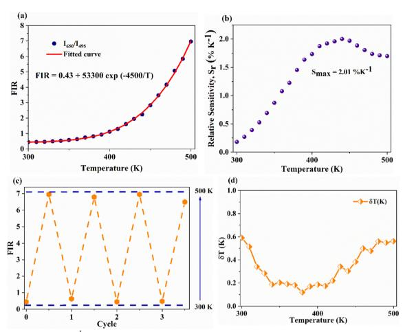
Fig. 7 (a) and (b) Variation of FIR $-\frac{I_{650}}{I_{495}}$  and relative sensitivity,  $S_r$  with temperature, (c) temperature cycling of FIR, and (d) the temperature resolution in the temperature range 300–500 K.
