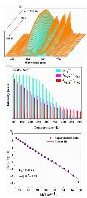
Fig. 5 (a) Temperature-dependent PL spectra of  $Sr_2NaMg_2-V_3O_{12}:0.05Sm^{3+}$  under 335 nm excitation, (b) the histogram showing the relative reduction in the intensity of dual emission from  $(VO_4)^{3-}$  and  $Sm^{3+}$  ions, and (c) linear fit of the Arrhenius equation.
