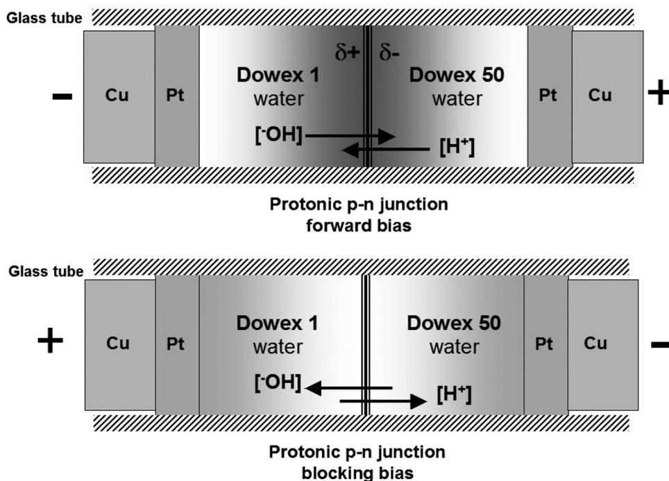
Fig. 1 Schematic diagram of the protonic p-n junction in action: the darkening in the middle corresponds to the variation in the density of the protons at the conductive (an increase) and blocking (a decrease) status, respectively.
