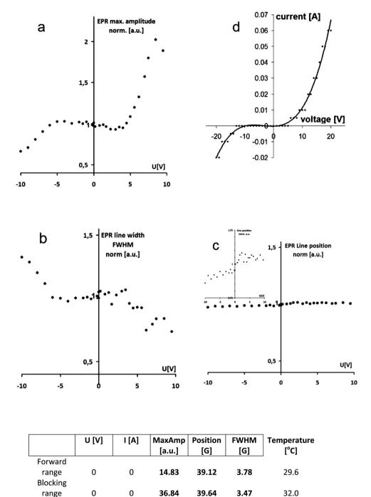
Fig. 3 Monitoring of the protonic p-n junction in action vs. bias voltage using L-band EPR and PANI EB as a spin probe: EPR signal amplitude (a), line width (b) and line position (c), and I-V characteristics of a protonic p-n junction composed of the same materials<sup>8</sup> (d) for comparison. The data set measured at a voltage of 0 V (direct read out) is presented in the table.
