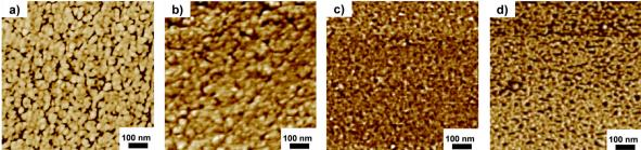
AFM phase images of PDPF-b-bisPip-2.0 (a), PDPF-b-bisPip-2.2 (b), PDPF-b-bisPip-2.4 (c) and PDPF-b-bisPip-2.6 (d)
