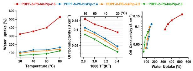
Fig. 4 Data of the AEMs in the fully hydrated hydroxide form: water uptake as a function of temperature (a), hydroxide conductivity as a function of  $T^{-1}$ (b), and hydroxide conductivity as a function of water uptake
