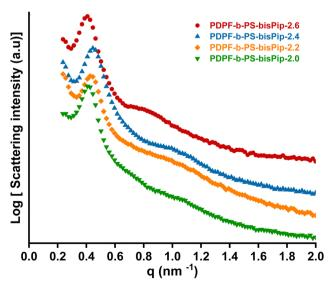
**Fig. 2** SAXS profiles of the BAB triblock copolymer AEMs in the PDPF-*b*-bisPip-IEC series in the dry bromide form.
