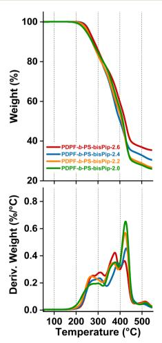
**Fig. 5** TGA traces of the triblock AEMs in the PDPF-*b*-PS-bisPip-IEC series (top) and the corresponding first derivatives (bottom).
