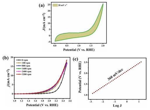
Fig. 6 Electro-chemical investigation of the OER in 1 M KOH solution (N2 saturated): (a) CV of the perovskite sample in the potential window of 0 to 2.0 V vs. RHE; (b) LSV graphs of ZTO at different rotations between the potentials of 0.0-2.4 V vs. RHE; (c) Tafel plot of ZTO.
