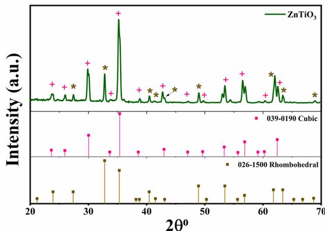
Fig. 1 XRD patterns of the as-prepared ZnTiO<sub>3</sub>.
