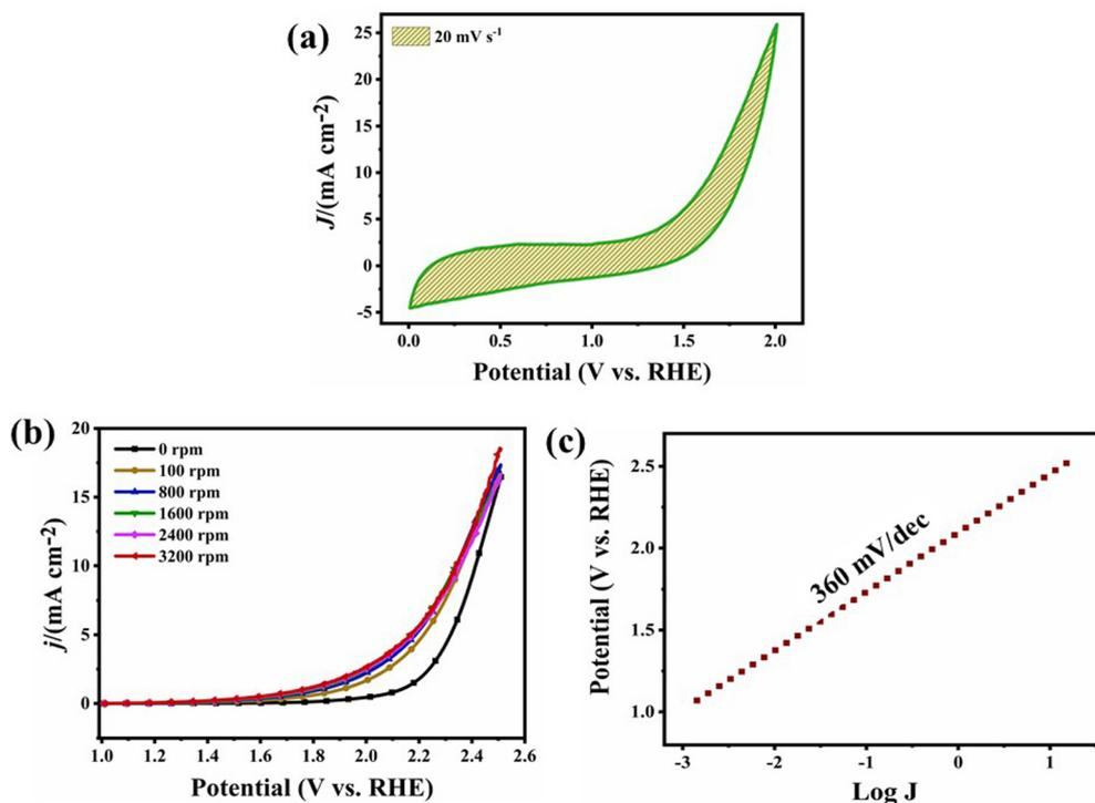
Fig. 6 Electro-chemical investigation of the OER in 1 M KOH solution (N<sub>2</sub> saturated): (a) CV of the perovskite sample in the potential window of 0 to 2.0 V vs. RHE; (b) LSV graphs of ZTO at different rotations between the potentials of 0.0–2.4 V vs. RHE; (c) Tafel plot of ZTO.
