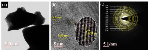
Fig. 4 (a and b) HRTEM images with interplanar spacing; (c) SAED pattern of ZTO.
