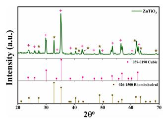
Fig. 1 XRD patterns of the as-prepared ZnTiO<sub>3</sub>
