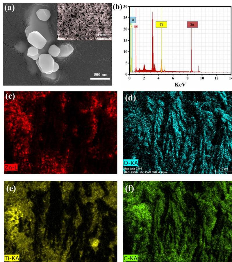
Fig. 3 EDS mapping and distribution of the as-prepared ZnTiO<sub>3</sub> (ZTO) slurry on the electrode: (a) FESEM image of the ZTO powder; (b) EDS spectra of ZTO; the distribution of the ZTO catalyst on Ni-foam, (c) Zn element (red), (d) O element (cyan), (e) Ti element (yellow), and (f) carbon element (green).
