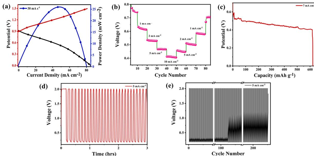
Fig. 8 Performance of the developed ZAB. (a) Polarisation curve with power density; (b) discharge curve at different scan rates of 1, 2, 5 and 10 mA cm<sup>-2</sup>; (c) discharge curve at the current density of 7 mA cm<sup>-2</sup>; (d) charge–discharge cycles; (e) battery voltage vs. cycle number.
