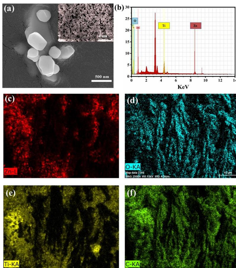
Fig. 3 EDS mapping and distribution of the as-prepared ZnTiO<sub>3</sub> (ZTO) slurry on the electrode: (a) FESEM image of the ZTO powder; (b) EDS spectra of ZTO; the distribution of the ZTO catalyst on Ni-foam, (c) Zn element (red), (d) O element (cyan), (e) Ti element (yellow), and (f) carbon element (green).
