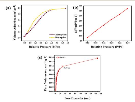
Fig. 5 (a) BET adsorption-desorption isotherms of the perovskite sample; (b) multi-point graph of ZnTiO<sub>3</sub>; (c) size distribution curve of ZnTiO<sub>3</sub> perovskite
