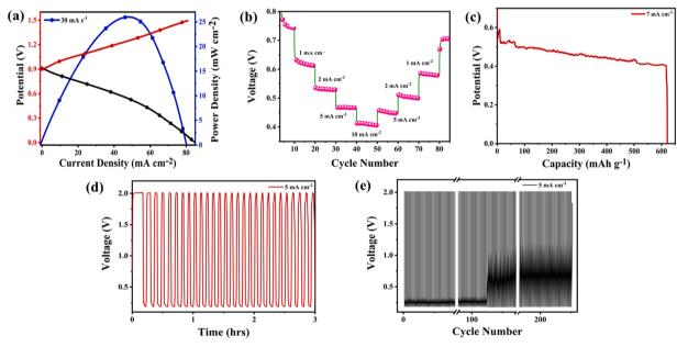
Fig. 8 Performance of the developed ZAB. (a) Polarisation curve with power density; (b) discharge curve at different scan rates of 1, 2, 5 and 10 mA cm<sup>-2</sup>; (c) discharge curve at the current density of 7 mA cm<sup>-2</sup>; (d) charge-discharge cycles; (e) battery voltage vs. cycle number.
