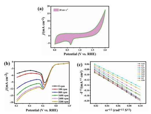
Fig. 7 ORR electro-chemical analysis in 0.1 M KOH solution, O<sub>2</sub> purged (a) CV of the perovskite sample in the potential window of 0 to 2 V vs. RHE; (b) RDE graphs of ZTO at different rotations in the potential range of 1 to 0.2 V vs. RHE; (c) Koutecky-Levich graph of the material at various potentials (V).
