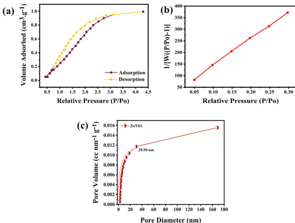
Fig. 5 (a) BET adsorption–desorption isotherms of the perovskite sample; (b) multi-point graph of  $ZnTiO_3$ ; (c) size distribution curve of  $ZnTiO_3$  perovskite.
