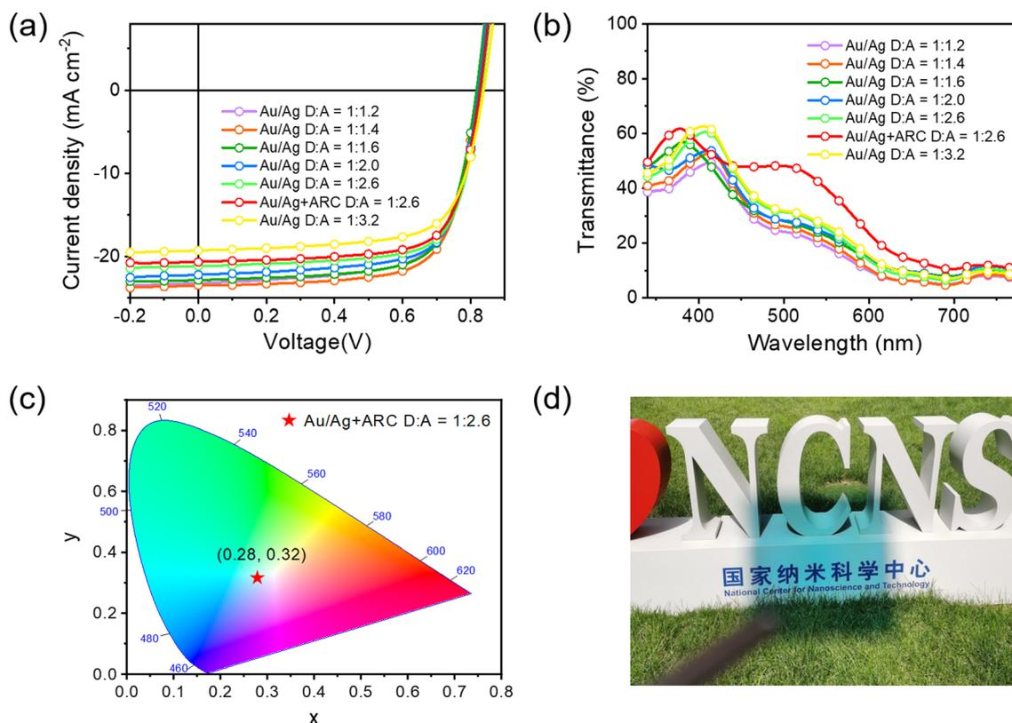
Fig. 5 (a)  $J$ - $V$  curves of PBDTTPTP:N3 semitransparent solar cells with different D/A ratios. (b) Transmittance spectra. (c) Coordinates of CIE 1931 for the best-LUE cell. (d) The photograph of a 1 cm<sup>2</sup> semitransparent cell made under optimal conditions.
