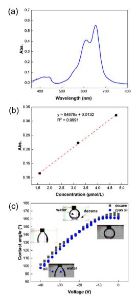
Fig. 3 (a) The UV-vis adsorption spectrum of cyan oil (8.2  $\times$  10<sup>-6</sup> M); (b) the molar extinction coefficient was  $64.876 \text{ L mol}^{-1} \text{ cm}^{-1}$ ; (c) the electrowetting curve of DI water drop in decane and cyan oil.
