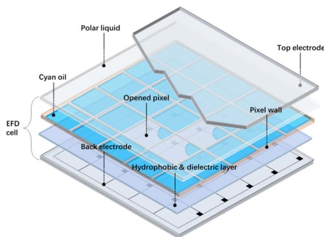
Fig. 1 Schematic drawing of the EFD cell structure.
