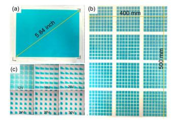
Fig. 6 Inkiet printing of **TDIC**. (a) 5.84 inch; (b)  $400 \times 500 \text{ mm}^2 \text{ EFD}$ devices; (c) opening pixels under different voltages.
