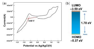
Fig. 4 (a) Cyclic voltammetry diagram of TDIC; (b) energy level diagram.
