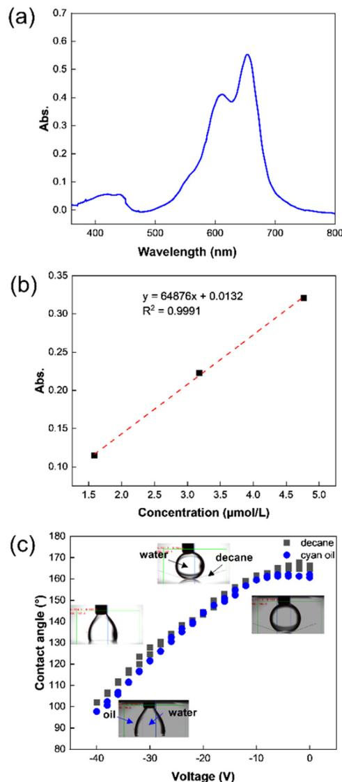
Fig. 3 (a) The UV-vis adsorption spectrum of cyan oil ( $8.2 \times 10^{-6} \text{ M}$ ); (b) the molar extinction coefficient was  $64876 \text{ L mol}^{-1} \text{ cm}^{-1}$ ; (c) the electro-wetting curve of DI water drop in decane and cyan oil.
