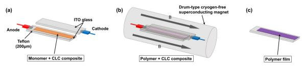
Fig. 1 Sandwich cell electrochemical polymerization in a liquid crystal under a magnetic field, and electrochemical polymerization in a CLC medium with transcription of its helical structure. CLC: cholesteric liquid crystal.
