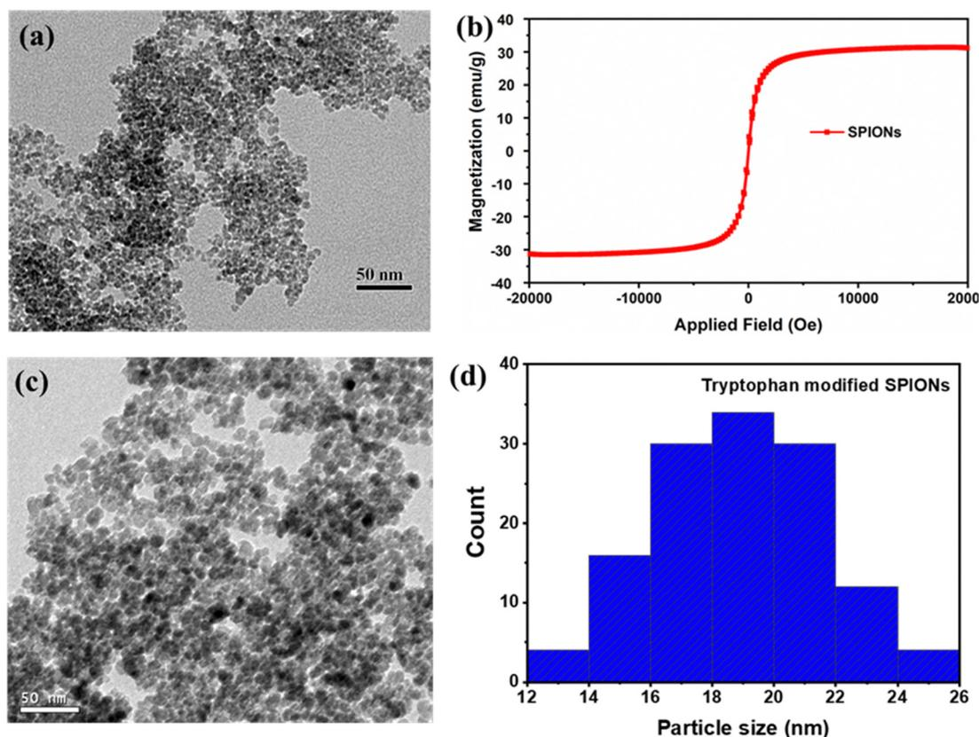
Fig. 1 (a) TEM image of pristine SPIONs, (b) magnetisation curve of pristine SPIONs studied at room temperature using VSM, (c) TEM image and (d) histogram of the particle size distribution of surface modified SPIONs using tryptophan.
