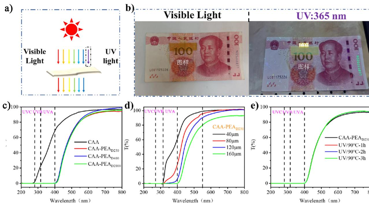
Fig. 3 (a) UV shielding schematic diagram, (b) photos of CAA-PEA<sub>D230</sub> film under UV (365 nm) and visible light, (c) UV-visible transmittance curves of CAA, CAA-PEA<sub>D230</sub>, CAA-PEA<sub>D400</sub>, and CAA-PEA<sub>D2000</sub> films, (d) UV-visible transmittance curves of CAA-PEA<sub>D230</sub> film with different thickness, and (e) UV-visible transmittance curves of the modified film irradiated with high power UV (365 nm) at 90 °C for different times.
