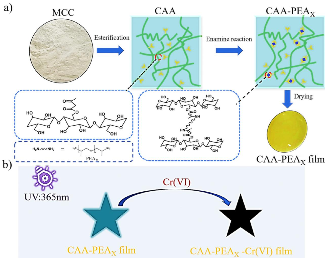
**Scheme 1** (a) Synthesis of the cross-linked cellulose-based film (CAA-PEA<sub>x</sub>), and (b) schematic diagram of fluorescence quenching of CAA-PEA<sub>x</sub> by Cr(vi) at 365 nm UV light.
