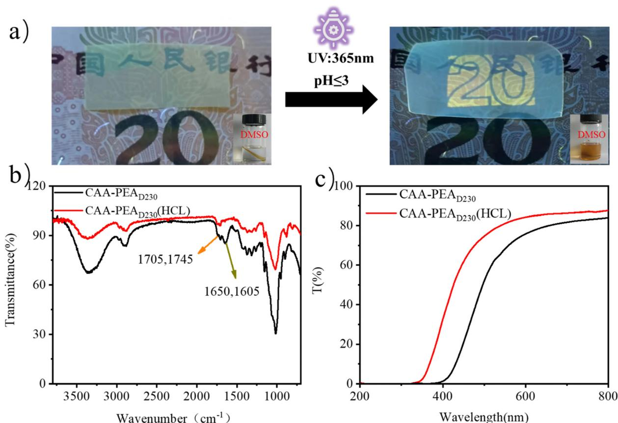
Fig. 4 (a) Photograph of UV shielding function and solubility of the film before and after HCl solution, (b) FT-IR spectra and (c) UV-visible transmittance curves of the film before and after acidolysis.
