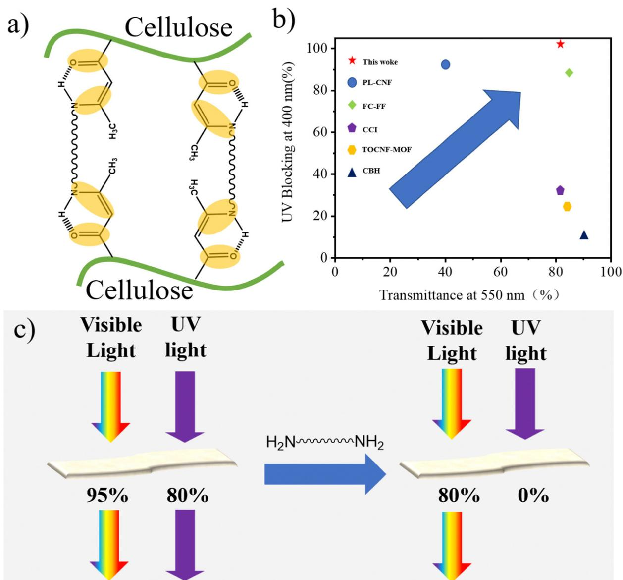
Fig. 5 (a) UV-blocking mechanism, (b) a comparison of the UV blocking and transparency of the CAA-PEA<sub>D230</sub> film with other Cellulose-based UV-shielding films, and (c) schematic showing the UV-filtering of the CAA-PEA film.
