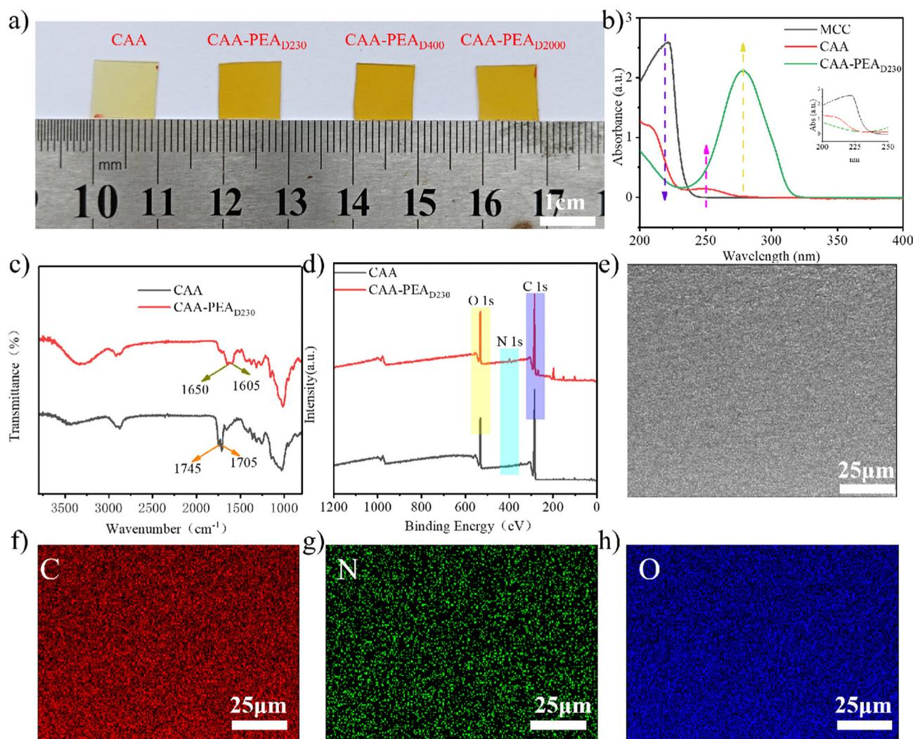
Fig. 1 (a) Optical images of cellulose acetoacetate film and film obtained by adding different polyether amines, (b) UV-vis absorption spectra of MCC, CAA and CAA-PEAx<sub>D230</sub> films, (c) FT-IR spectra and (d) XPS wide-scan spectra of the CAA film and the CAA-PEAx<sub>D230</sub> film, (e) SEM diagrams of cross sections of the CAA-PEAx<sub>D230</sub> film, (f–h) EDS elemental mapping images C, N, O of the CAA-PEAx<sub>D230</sub> film.
