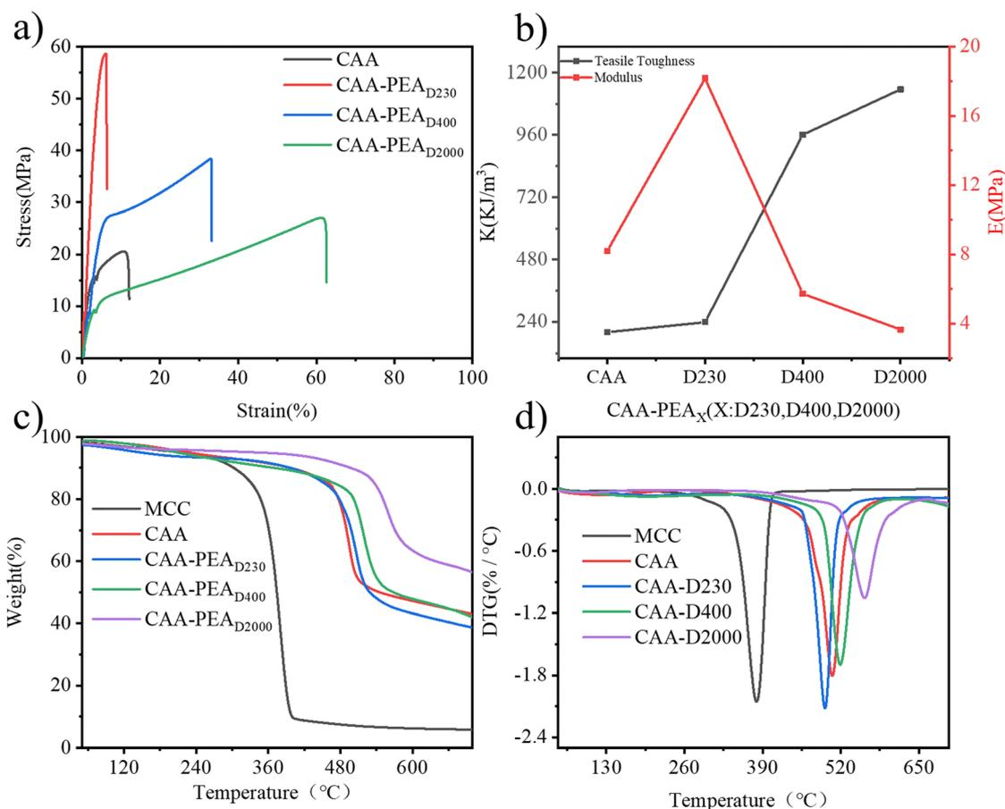
Fig. 2 Characterization and properties of the film: (a) stress-strain curves (b) corresponding mechanical parameters (c) TG and (d) DTG curves of the cellulose, CAA film, and CAA-PEA<sub>x</sub> film.
