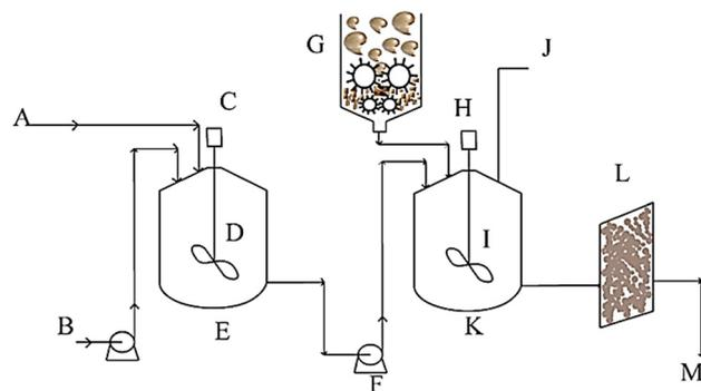
**Scheme 1** Process flow diagram for the synthesis of triple superphosphate. Notations: A = 85% H<sub>3</sub>PO<sub>4</sub> inlet, B = deionized water inlet pump, C = motor, D = stirrer, E = vessel for acid dilution, F = 60% acid inlet pump, G = ball mill, H = motor, I = stirrer, J = CO<sub>2</sub> vent, K = main reactor, L = drying unit, M = final product.
