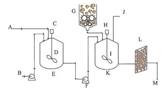
Scheme 1 Process flow diagram for the synthesis of triple superphosphate. Notations: A = 85% H<sub>3</sub>PO<sub>4</sub> inlet, B = deionized water inlet pump, C = motor, D = stirrer, E = vessel for acid dilution, F = 60% acid inlet pump, G = ball mill, H = motor, I = stirrer, J = CO2 vent, K = main reactor, L = drying unit, M = final product.
