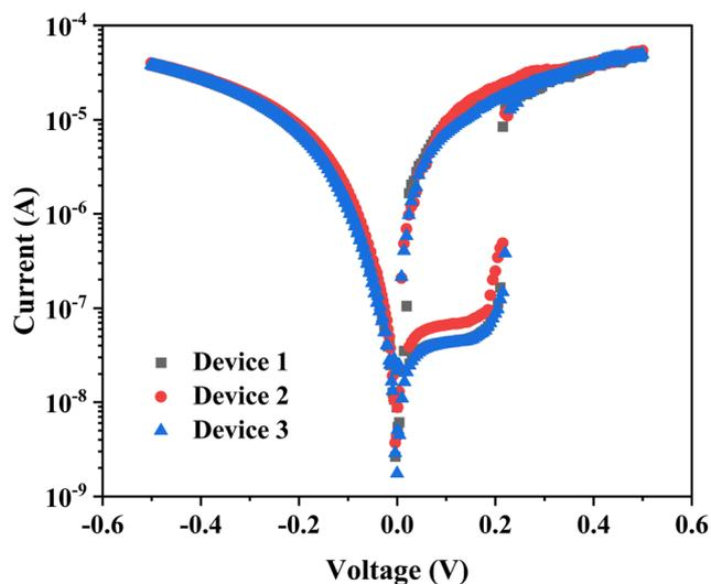
Fig. 7 Device-to-device variation of Cu/Cu<sub>2</sub>S/DNA/Au junctions.
