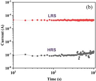
Fig. 6 Typical (a) endurance and (b) retention performance of the Cu/Cu₂S/DNA/Au junction.
