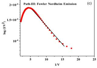
Fig. 9 The experimental data of the Cu/Cu<sub>2</sub>S/DNA/Au junction fitted to various charge-transport mechanisms: (a) Schottky-barrier emission, (b) Poole-Frenkel emission and (c) direct Fowler-Nordheim tunneling. The solid lines show the best fit to the experimental data points.
