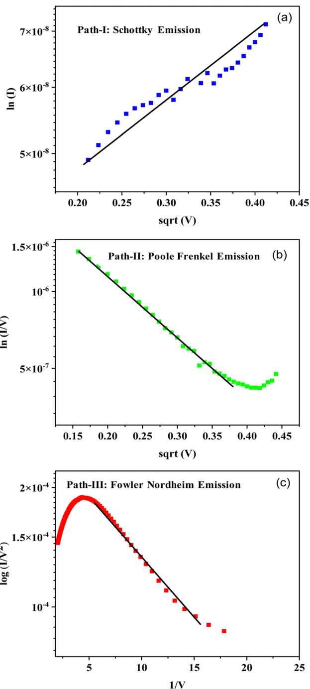
Fig. 9 The experimental data of the Cu/Cu<sub>2</sub>S/DNA/Au junction fitted to various charge-transport mechanisms: (a) Schottky-barrier emission, (b) Poole–Frenkel emission and (c) direct Fowler–Nordheim tunneling. The solid lines show the best fit to the experimental data points.
