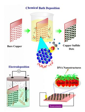
Fig. 1 Schematic illustration of electroless and electrochemical syntheses of  $\text{Cu}_2\text{S}$  and DNA on the Cu substrate and finally the constitution of the  $\text{Cu}/\text{Cu}_2\text{S}-\text{DNA/Au}$  junction.
