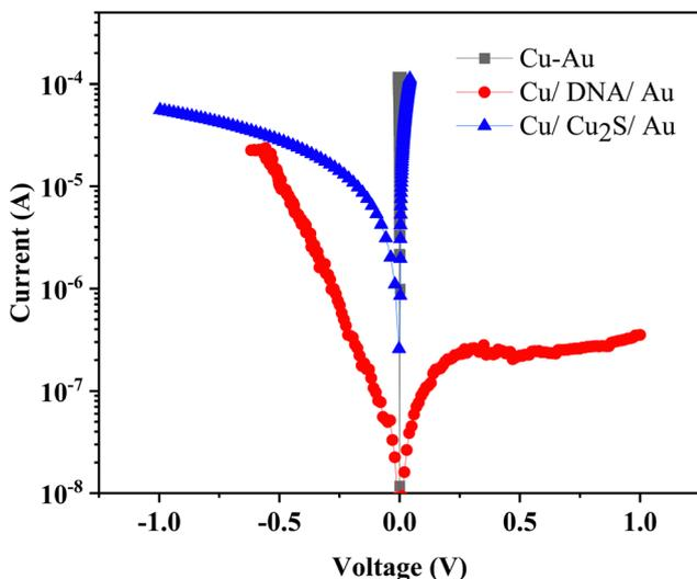
Fig. 4 Comparison of  $I$ - $V$  curves of Cu/Au, Cu/DNA/Au and Cu/Cu<sub>2</sub>S/Au junctions.
