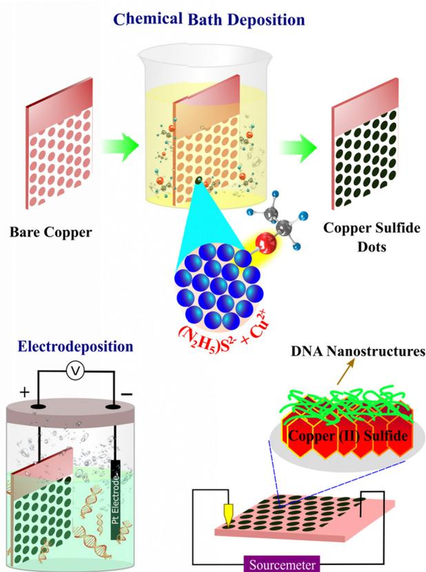
Fig. 1 Schematic illustration of electroless and electrochemical syntheses of  $\text{Cu}_2\text{S}$  and DNA on the Cu substrate and finally the constitution of the  $\text{Cu}/\text{Cu}_2\text{S}$ -DNA/Au junction.
