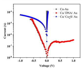
Fig. 4 Comparison of I-V curves of Cu/Au, Cu/DNA/Au and Cu/Cu<sub>2</sub>S/Au iunctions
