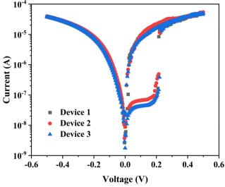
Fig. 7 Device-to-device variation of Cu/Cu<sub>2</sub>S/DNA/Au junctions.
