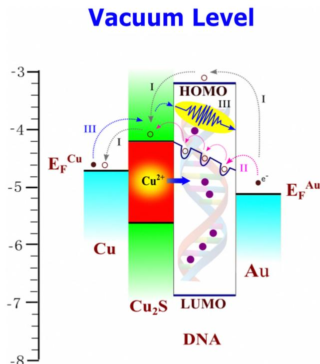
Fig. 8 Energy-band diagram of the Cu/Cu<sub>2</sub>S/DNA/Au junction, indicating various paths of charge transport.
