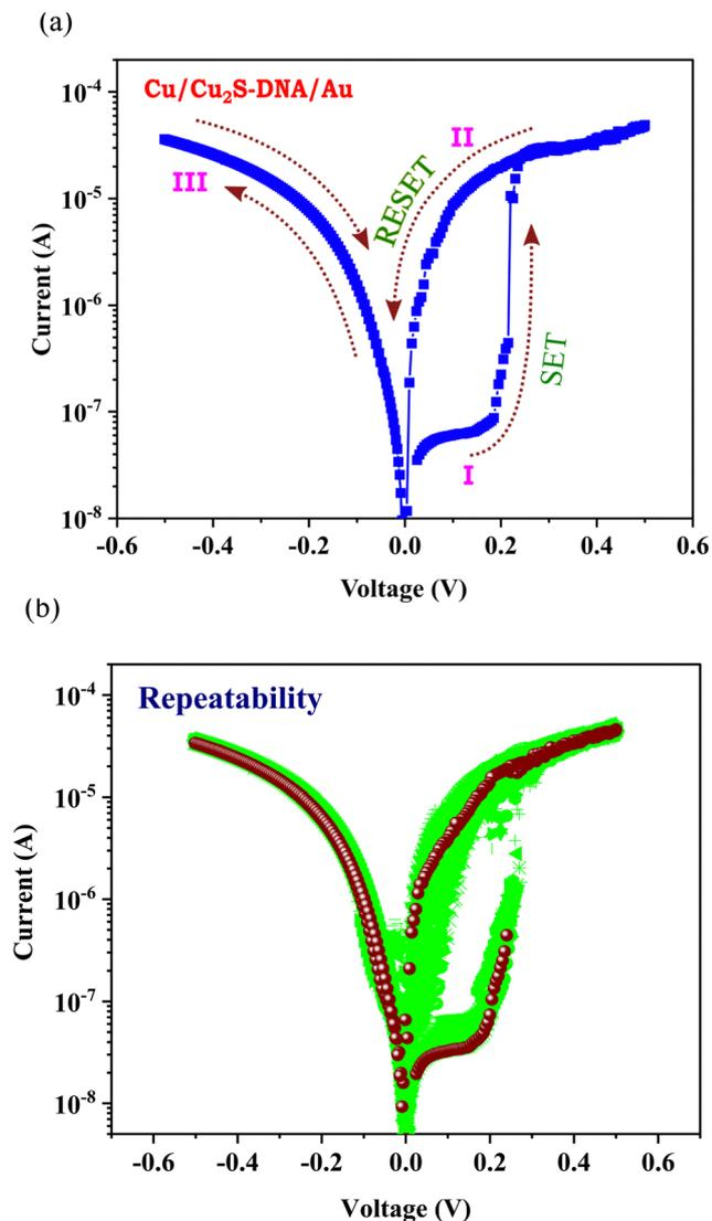
Fig. 5 (a) Memristor current–voltage curve of Cu/Cu<sub>2</sub>S/DNA/Au junction, here arrows show directions of scan. (b) Repeatability curves of a junction for 30 cycles.
