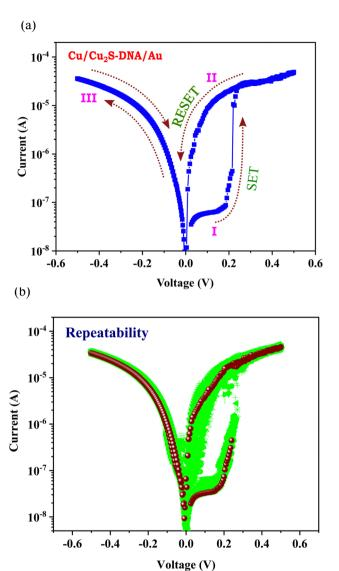
Fig. 5 (a) Memristor current–voltage curve of  $\text{Cu/Cu}_2\text{S/DNA/Au}$  junction, here arrows show directions of scan. (b) Repeatability curves of a junction for 30 cycles.
