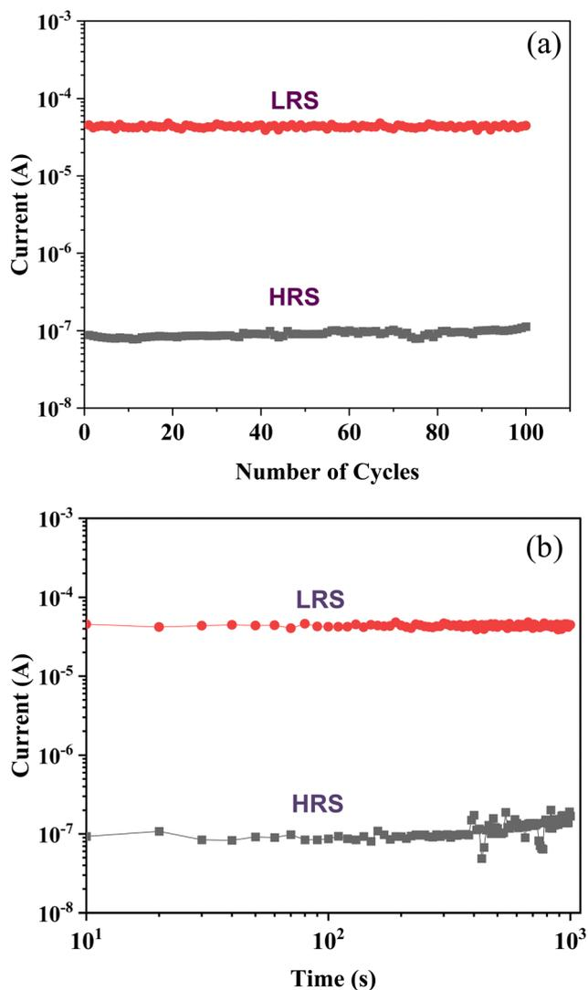
Fig. 6 Typical (a) endurance and (b) retention performance of the Cu/Cu<sub>2</sub>S/DNA/Au junction.
