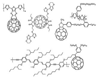
Fig. 33 Covalent linkages of conducting polymers onto fullerenes; reprinted with permission from ref. 273; copyright © Royal Society of
