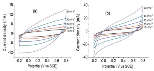
Fig. 30 CV loops of (a) single layer PPy/AC supercapacitor electrodes and (b) multilayer supercapacitor electrodes; reprinted with permission from ref. 249; copyright @ Taylor & Francis Group
