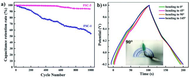
Fig. 24 (a) Cycling behavior of FSC-1 and FSC-5 asymmetric supercapacitors. (b) GCD curves of FSC-5 with different bending angles at a current density of 1 mA cm<sup>-2</sup>; reprinted with permission from ref. 202; copyright © Royal Society of Chemistry.
