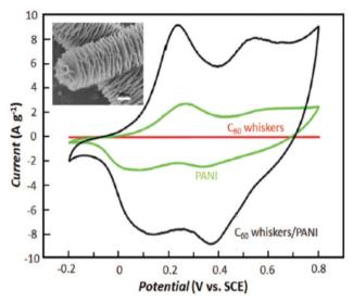
Fig. 35 Cyclic voltammogram of  $C_{60}$ , polyaniline and their nanocomposites; the SEM image of the nanocomposites is shown in the inset; reprinted with permission from ref. 279; copyright © Elsevier.
