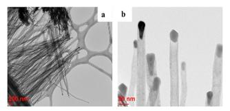
Fig. 11 TEM images of CNTs grown on the CNT sheet by PECVD; reprinted with permission from ref. 131; copyright © Elsevier.
