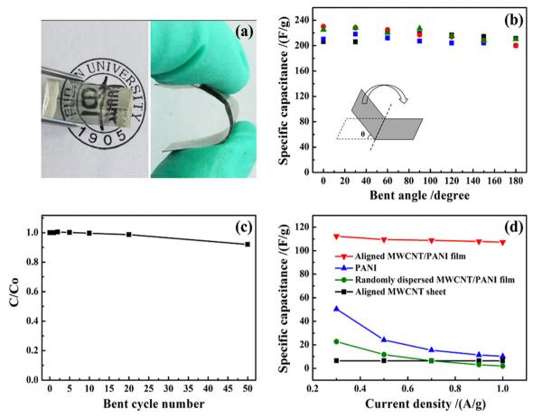
Fig. 13 (a) A typical PANI/multiwalled CNT flexible nanocomposite film.(b) Variation of specific capacitance with the bending angle. (c) Dependence of the ratio of specific capacitance of the system before and after bending versus the bending cycle number. (d) Variation of specific capacitance with current density; reprinted with permission from ref. 132; copyright © Springer Nature.
