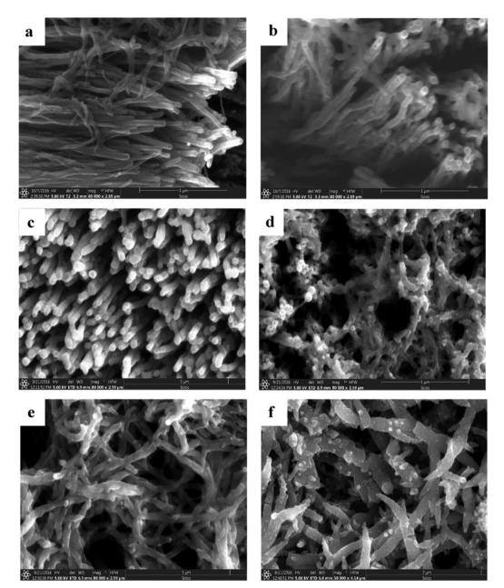
Fig. 12 (a-e) SEM images of PANI/CNT after 10, 20, 30, 40 and 50 cycles of PANI deposition. (f) SEM image of the PANI/pristine CNT sheet after 30 cycles of PANI deposition; reprinted with permission from ref. 131; copyright © Elsevier.
