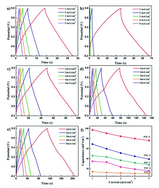
Fig. 23 GCD profiles of (a) PPy, (b) PPy-GO 1, (c) PPy-GO 1.5, (d) PPy-GO 2 and (e) PPy-GO 2.5 at different current densities. (f) Plots of areal specific capacitance for FSCs (FSCs: flexible supercapacitors, FSC-1 = PPy, FSC-2 = PPy-GO 1, FSC-3 = PPy-GO 1.5, FSC-4 = PPy-GO 2, and FSC-5 = PPy-GO 2.5); reprinted with permission from ref. 202; copyright © Royal Society of Chemistry.
