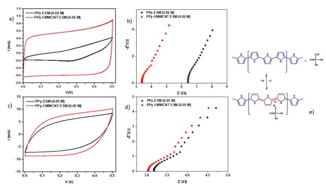
Fig. 18 Voltammograms of PPy/egg shell membranes and PPy/CNT/egg shell membranes by using (a) 0.02 M PPy and (c) 0.05 M PPy; the corresponding impedance spectrum at 50 mV s<sup>-1</sup> using (b) 0.02 M PPy and (d) 0.05 M PPy; (e) charge storage mechanism of CNT/PPy in  $H_3PO_4/PVA$  systems; reprinted with permission from ref. 144; copyright © American Chemical Society.
