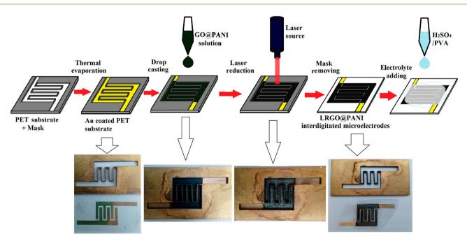
Fig. 20 Schematic and digital photograph of fabrication of PANI/RGO microcapacitor electrodes; reprinted with permission from ref. 198; copyright (i) American Chemical Society
