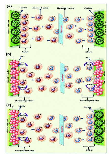
Fig. 2 A schematic representation of the reaction mechanism between an alkaline electrolyte (KOH) and a representative electrode: (a) electrical double layer capacitor, (b) pseudocapacitor, and (c) hybrid supercapacitor; reprinted with permission from ref. 20; copyright © Royal Society of Chemistry.
