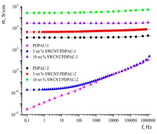
Fig. 9 Frequency dependence of conductivity for PDPAC and SWCNT/ PDPAC nanocomposites; reprinted with permission from ref. 122; copyright @ MDPI.
