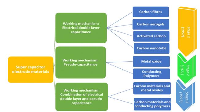
Fig. 3 Taxonomy and timeline of supercapacitor materials.
