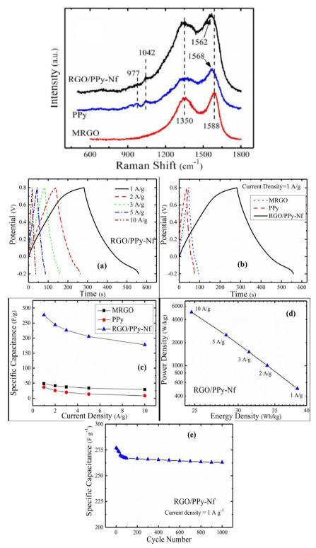
Fig. 26 (a) Raman spectra of MRGO, PPy, and the RGO/PPy-NF nanocomposite; reprinted with permission from ref. 204; copyright © Springer. (b) (a) GCD plot of the RGO/PPy nanocomposite with current density. (b) GCD plot of the samples at a current density of 1 A g<sup>-1</sup>. (c) Variation of specific capacitance with current density. (d) Ragone plot. (e) Specific capacitance vs. cycle numbers for the RGO/PPy nanocomposite; reprinted with permission from ref. 204; copyright © Springer.
