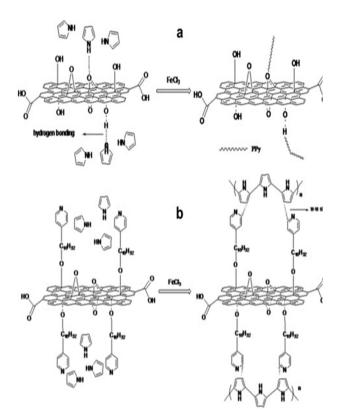
Fig. 25 Possible combining mode of (a) PPy/GO and (b) PPy/modified GO; reprinted with permission from ref. 203; copyright © Elsevier.
