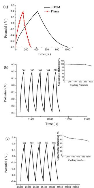
Fig. 17 (a) Galvanostatic charge/discharge curves of planar PPy/CNT nanocomposites and PPy/3 DMO nanocomposites. (b) Continuous galvanostatic charge/discharge curves of planar PPy/CNT nanocomposites after 500 cycles. (c) Charge-discharge curves of 3 DOM-PPy/CNT nanocomposite supercapacitor electrodes after 500 cycles; reprinted with permission from ref. 142; copyright © American Chemical Society.
