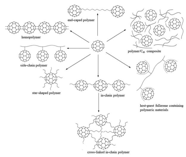
Possible structures formed by the incorporation of polymers onto fullerenes; reprinted with permission from ref. 268; copyright © Wiley Online Library
