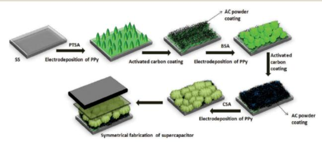
Fig. 29 A schematic representation of PPy/AC nanocomposite supercapacitor electrode fabrication; reprinted with permission from ref. 249; copyright @ Taylor & Francis Group [SS: stainless steel].
