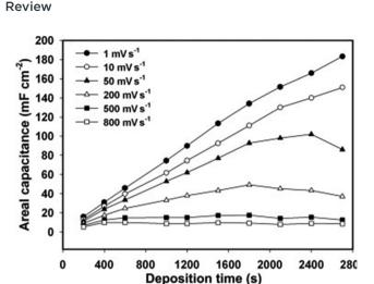
Fig. 27 Areal capacitance versus deposition time plot of RGO/PPy electrodes with different CV scan rates; reprinted with permission from ref. 208; copyright © Elsevier.
