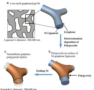
Fig. 31 Schematic representation of fabrication of graphene/PPy nanocomposites; reprinted with permission from ref. 262; copyright @ Elsevier.
