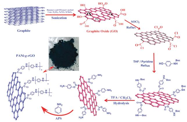
Fig. 22 Schematic representation of the synthesis of PANI-g-GO nanocomposites; reprinted with permission from ref. 200; copyright © American Chemical Society
