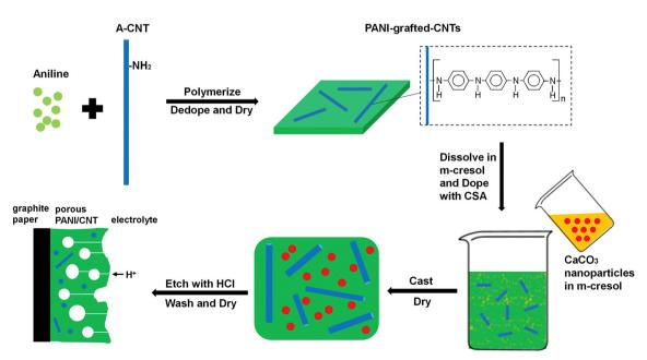
Fig. 14 Schematic representation of synthesis of porous PANI/CNT electrodes; reprinted with permission from ref. 133; copyright © Elsevier.
