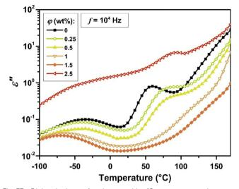
Fig. 37 Dielectric loss of polyazomethine/ $C_{60}$  nanocomposites as a function of temperature; reprinted with permission from ref. 282; copyright © Elsevier.
