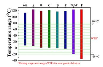
Fig. 4 Effect of target compounds on the temperature range of LC mixtures. Each of five compounds **4TV**, **4FTV**, **4FTFV** and **2TFV** (15 wt%) was dissolved in LC mixture **001**, yielding new LC mixtures **A**, **B**, **C**, **D** and **E**. Compound **2TFV** (15 wt%) was dissolved in the LC mixture **P02-F**, yielding new LC mixture **F**.
