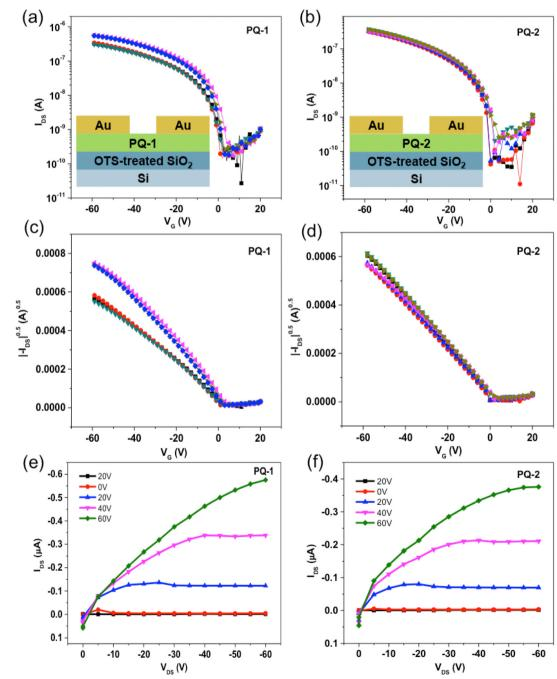
Fig. 6 (a) Transfer, (c)  $|I_{DS}|^{1/2}$ - $V_G$ , and (e) output curves of OFETs based on **PQ-1**; (b) transfer, (d)  $|I_{DS}|^{1/2}$ - $V_G$  and (f) output curves of OFETs based on **PQ-2**.
