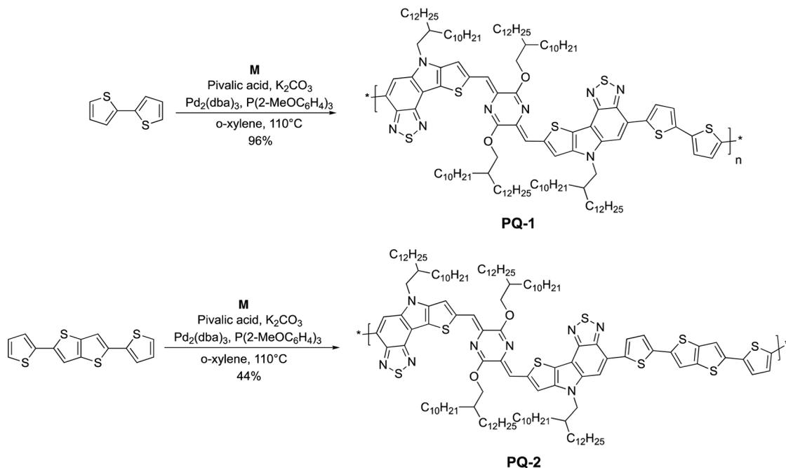
Scheme 2 Synthesis of the polymers **PQ-1** and **PQ-2**.Table 1 Molecular weights and polydispersity index (*D*) of **PQ-1** and **PQ-2**
