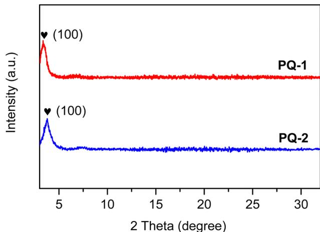
Fig. 7 X-ray diffraction patterns of PQ-1 and PQ-2.
