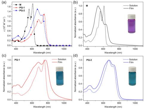
Fig. 4 (a) UV-vis absorption spectra of the chlorobenzene solutions of M, PQ-1 and PQ-2; (b-d) Normalized UV-vis absorption spectra of the chlorobenzene solutions and thin films of M, PQ-1 and PQ-2.
