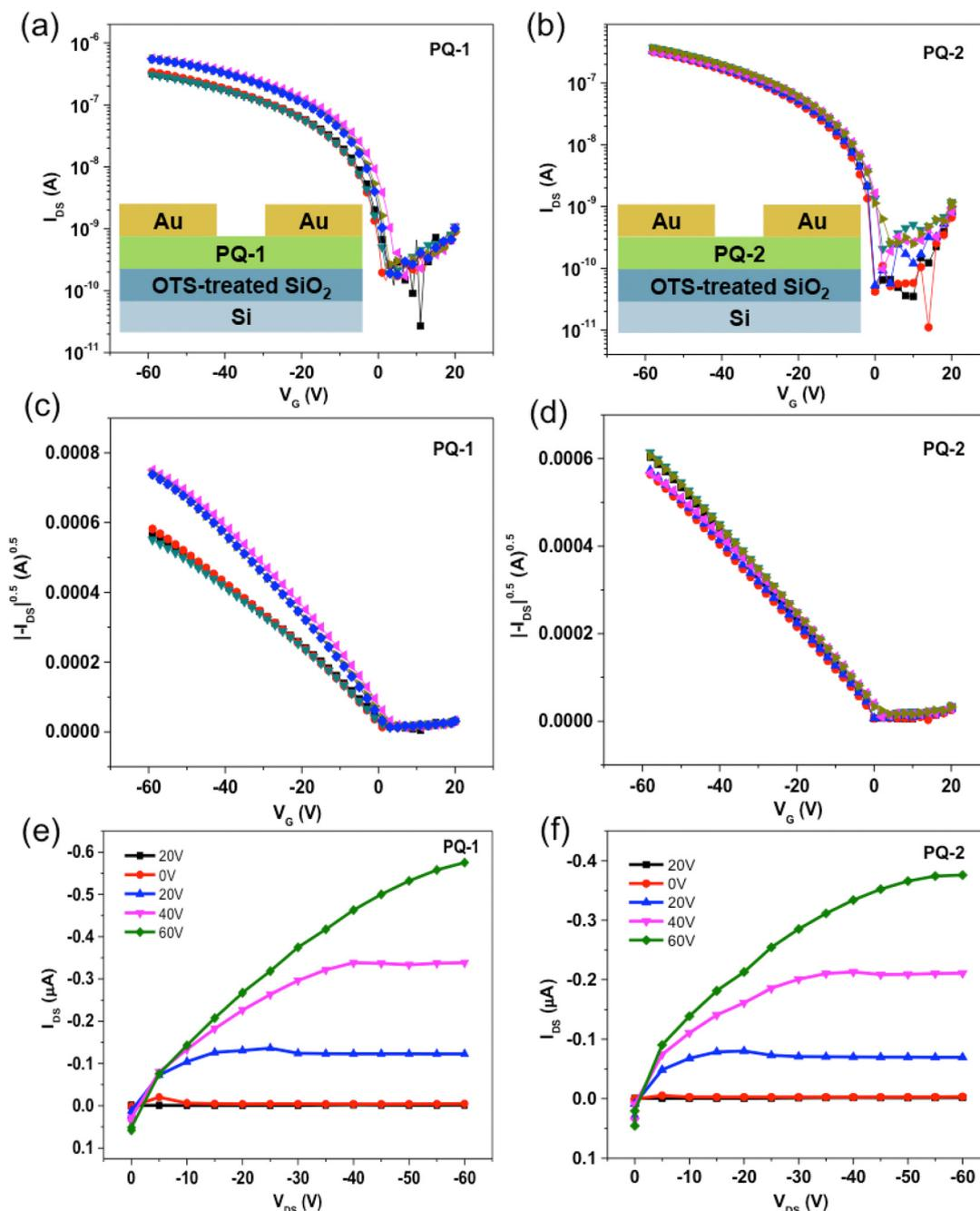
Fig. 6 (a) Transfer, (c)  $|I_{\text{DS}}|^{1/2}$ - $V_{\text{G}}$ , and (e) output curves of OFETs based on **PQ-1**; (b) transfer, (d)  $|I_{\text{DS}}|^{1/2}$ - $V_{\text{G}}$  and (f) output curves of OFETs based on **PQ-2**.
