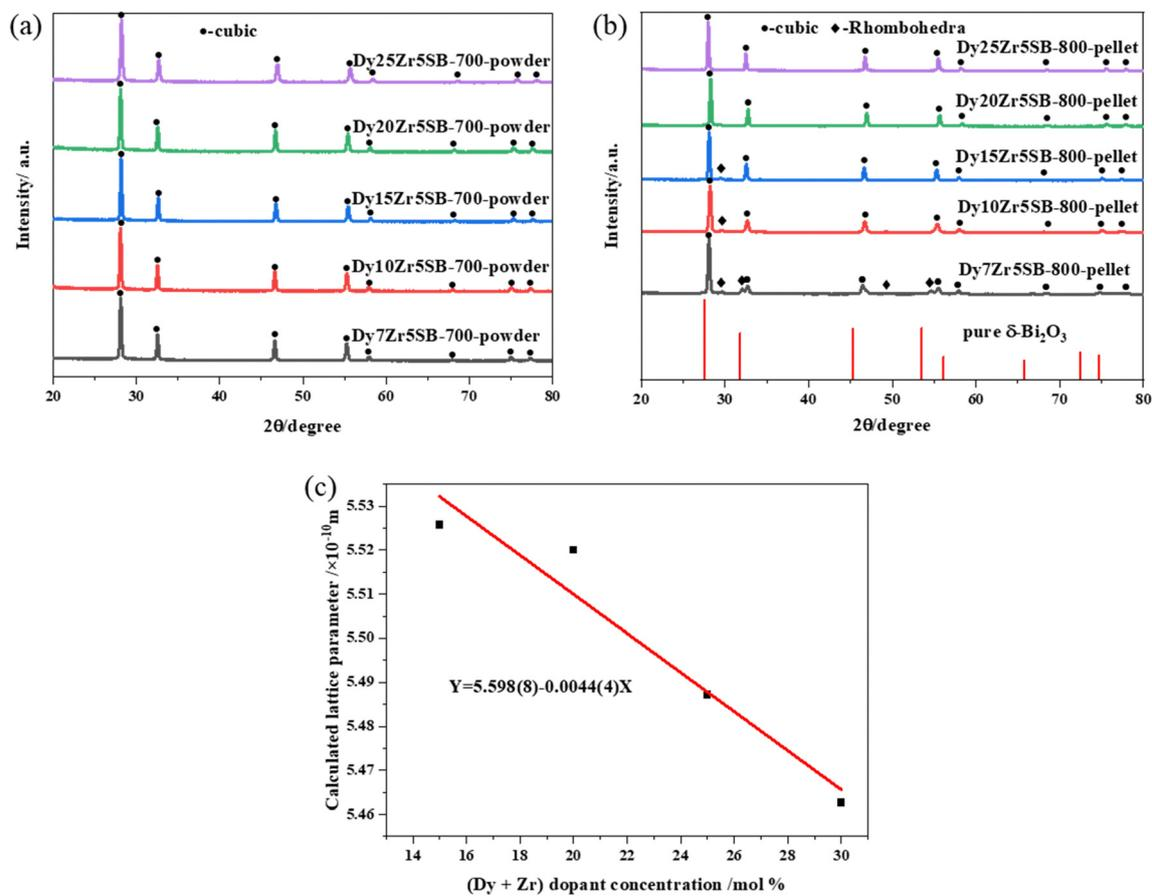
Fig. 5 XRD patterns of  $\text{Dy}_x\text{Zr}_{0.05}\text{Bi}_{0.95-x}\text{O}_{1.5-\delta}$ . (a) powders calcined at 700 °C for 2 h, (b) pellets sintered at 800 °C for 5 h and (c) effects of total dysprosium and zirconium dopant concentrations (mol%) on the lattice parameters estimated using the Rietveld analysis.
