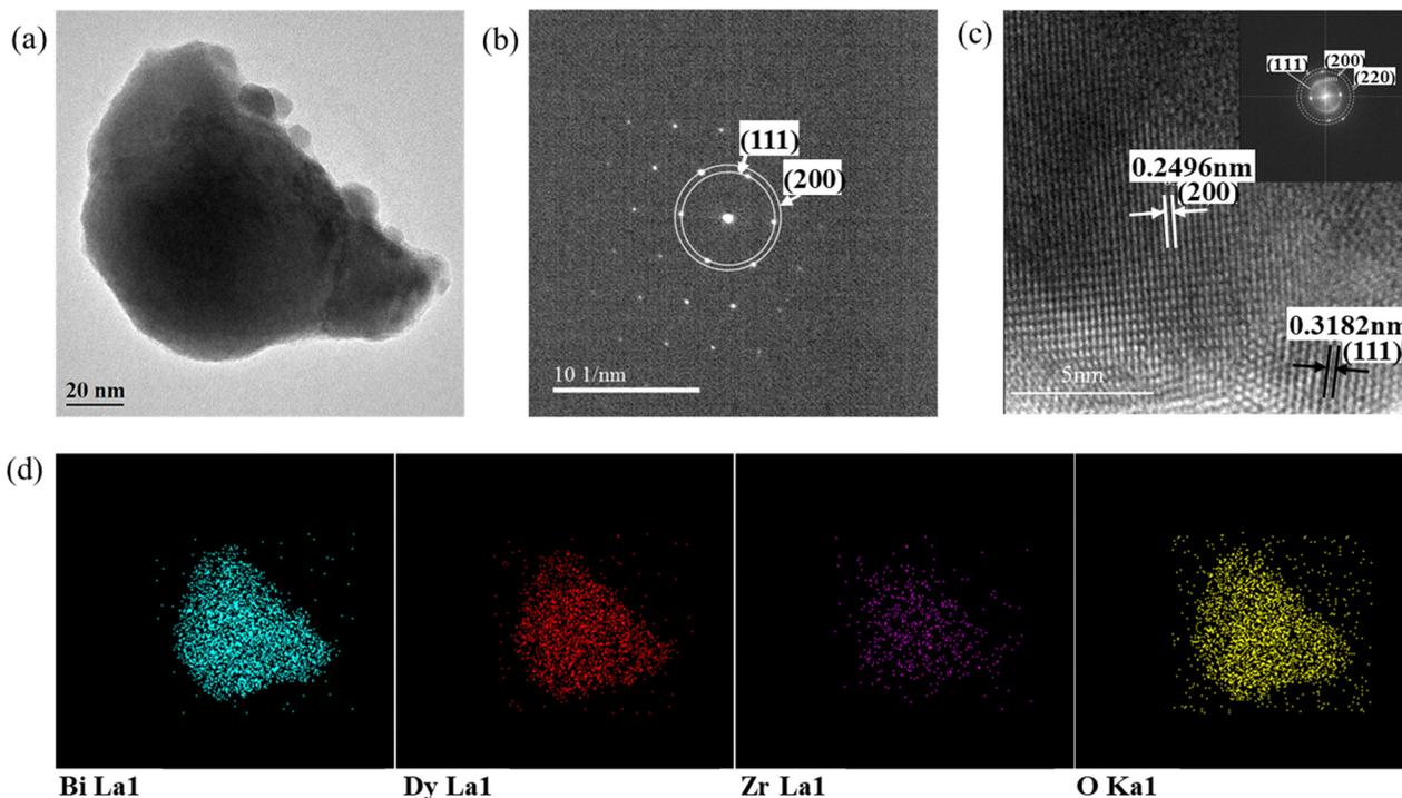
Fig. 6 HR-TEM images of  $\text{Bi}_{0.75}\text{Dy}_{0.20}\text{Zr}_{0.05}\text{O}_{1.5-\delta}$ . (a) Bright-field image. (b) SAED pattern obtained from area displayed in Fig. 6(a). (c) Nanocrystalline fringe pattern and inserted Fast Fourier Transform (FFT) of a selected zone of the fringe pattern. (d) EDS mapping.
