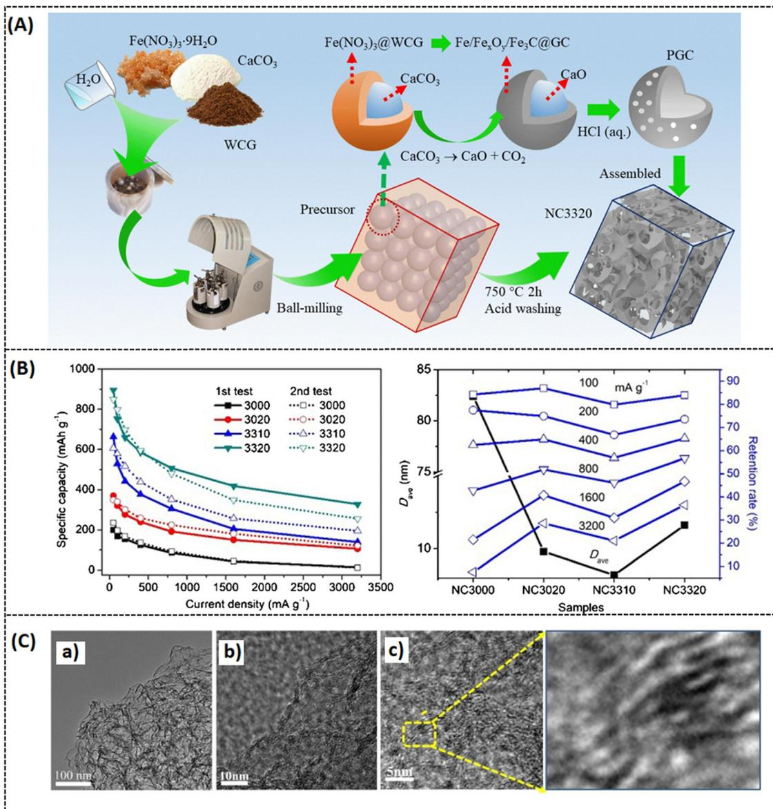
Fig. 3 (A) Schematic representation of porous carbon network, (B) capacitance at different current densities from 50 to 3200  $\text{mA g}^{-1}$ , (d) comparative response of retention rate vs.  $D_{\text{ave}}$  of different samples at various current densities, (C) TEM images of the optimal sample at different magnifications. Reprinted with permission,<sup>40</sup> Copyright (2021) from Elsevier.
