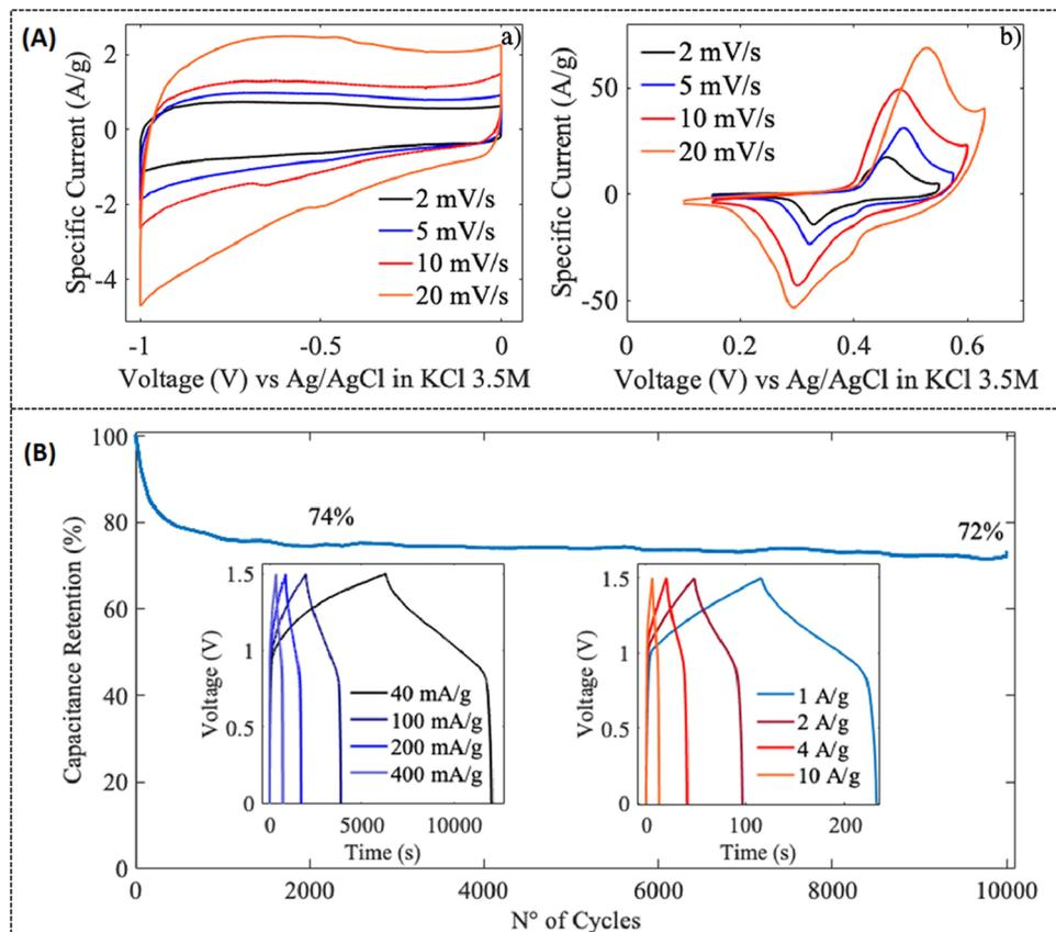
Fig. 16 (A) (a and b) CV response of TEGO and Ni-TEGO at different scan rates, (B) capacitance retention response of ASCs over 10 000 cycles at  $1 \text{ A g}^{-1}$  current density inset: with GCD curves at different applied current density. Reprinted with permission,<sup>97</sup> Copyright (2022) from Elsevier.
