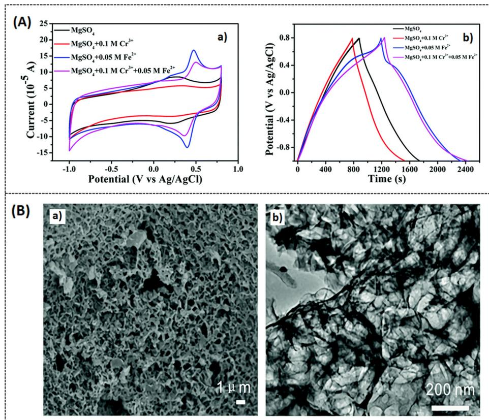
Fig. 15 (A) (a and b) CV response of optimal composite BPGC at different electrolyte medium at a scan rate 5 mV s<sup>-1</sup>, GCD response at 0.5 A g<sup>-1</sup> current density. (B) (a and b) SEM and TEM images of BPGC. Reproduced with permission,<sup>96</sup> Copyright (2022), Royal Society of Chemistry.
