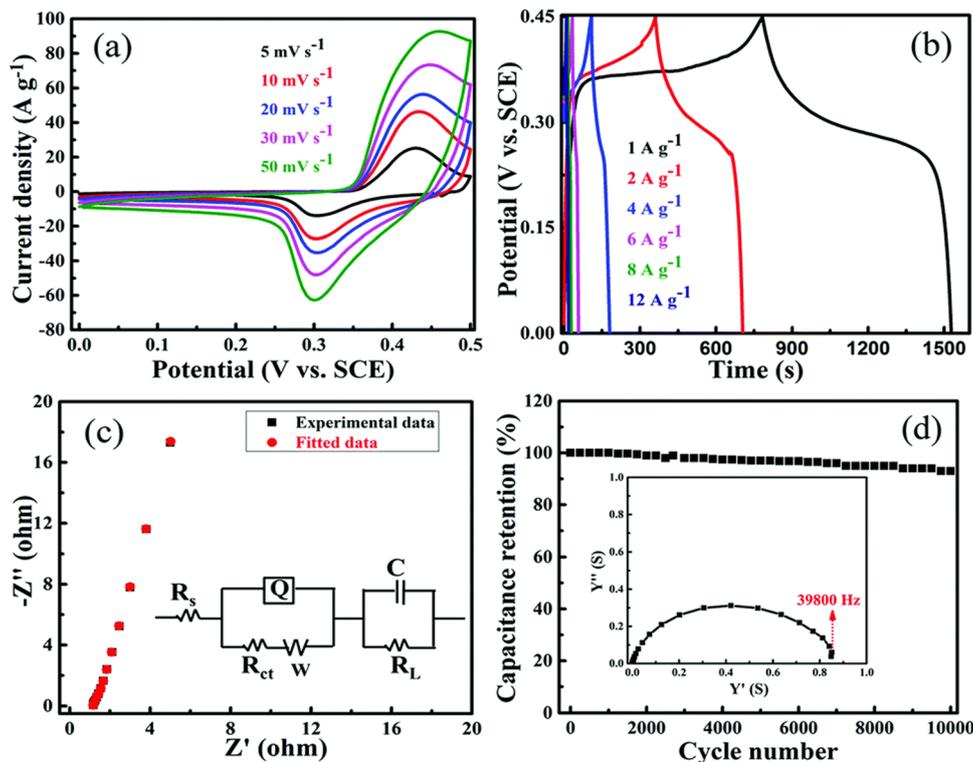
Fig. 12 Electrochemical responses of 10 PGNC composite (a–d) CV curves at different scan rates, GCD at different applied current densities, Impedance plot, cycling stability at  $8 \text{ A g}^{-1}$  with admittance plot. Reproduced with permission,<sup>92</sup> Copyright (2020), Royal Society of Chemistry.
