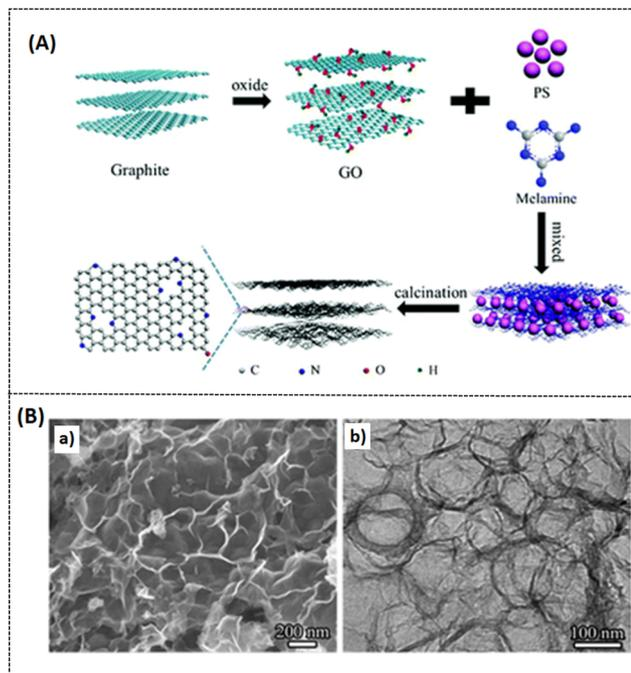
Fig. 10 (A) Schematic representation of preparation protocol of N-3DPG, (B) (a and b) FE-SEM and TEM images of N-3DPG. Reproduced with permission,<sup>72</sup> Copyright (2017), Royal Society of Chemistry.
