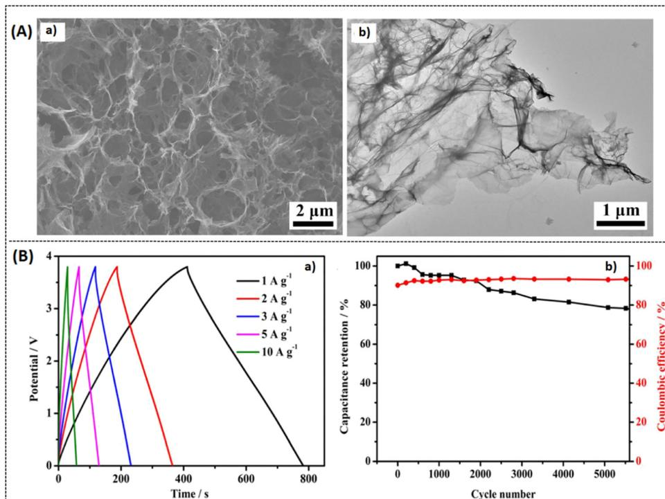
Fig. 13 (A) SEM images of (a) UPGA and (b) TEM image of UPGA, (B) electrochemical Response of UPGA: (a) GCD response (b) cycling stability vs. coulombic efficiency at  $1 \text{ A g}^{-1}$ . Reprinted with permission,<sup>93</sup> Copyright (2021) from Elsevier.
