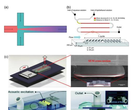
Fig. 4 Different microfluidic methods. (a) Schematic of hydrodynamic flow focusing. (b) Schematic of staggered herringbone micromixer. (c) Acoustic micromixing devices using star-shaped oscillating plates: the assembled star-shaped microfluidic mixer (top) and the ultrafast star-shaped acoustic micromixer (bottom). The figure is adopted from ref. 39 with permission.
