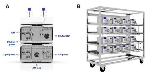
Fig. 3 IJM devices used in the laboratory (A) and industry (B). This figure is adopted from ref. 32 with permission.
