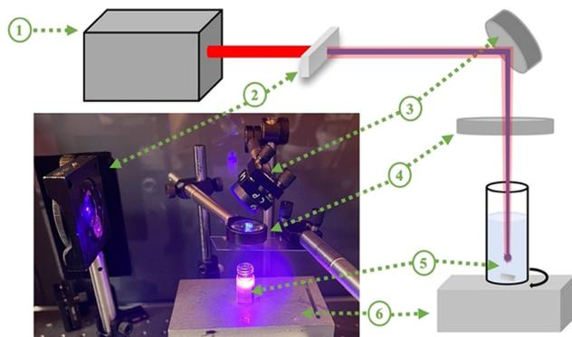
Fig. 1 Schematic representation and photograph of the laser irradiation experiment setup containing the (1) Ti:sapphire pulsed laser, (2) barium borate (BBO) non-linear crystal, (3) mirror, (4) focus lens ( $f = 50$  mm), (5)  $\text{TiO}_2$  dispersion with a magnetic stir bar, and (6) magnetic stirrer.
