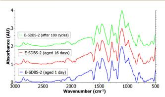
Fig. 8 IR spectra of pristine E-SDBS-2, 16 days aged E-SDBS-2 and E-SDBS-2 after cycling with CV.
