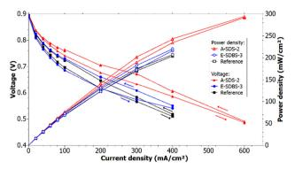
Fig. 12 Recorded polarization curves at a RH of 50% and the calculated power density
