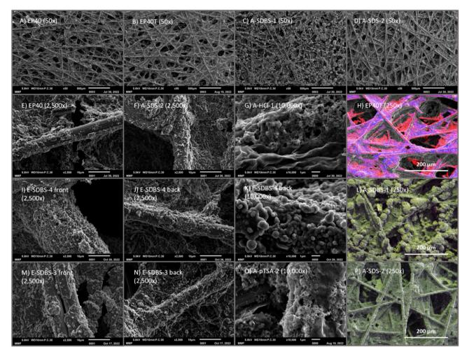
Fig. 10 SEM images of coated CP with magnification 50×, 2500× and 10 000× and EDX mapping of the investigated samples and the reference (color code is depicted in Table 5, for simplicity carbon is not shown in the PANI-coated samples). Additional SEM & EDX images are shown in ESI,† Fig. S10.
