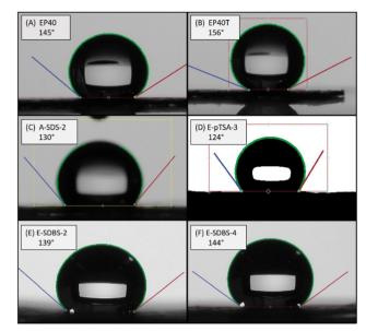
**Fig. 9** Highest contact angle determined for (A) EP40, (B) EP40T, (C) A-SDS-2, (D) E-pTSA-3, (E) E-SDBS-2 and (F) E-SDBS-4. The value depicted is the average of the contact angle on the left and on the right side of the drop
