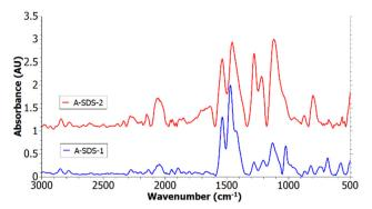
Fig. 6 IR spectra of A-SDS-1 (alkaline synthesis) and A-SDS-2 (acidic
