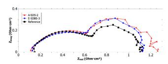
Fig. 11 Nyquist plot of EIS measurement with 280 mA cm<sup>-2</sup> and 50% RH.
