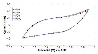
Fig. 4 Multi-scan cyclic voltammogram of E-SDBS-2 in 0.1 M HCl measured over a potential range of 0.4–0.95 V vs. RHE, 100 cycles with a scan rate of 20 mV s<sup>-1</sup>.
