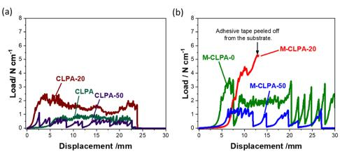
Fig. 3 Load-displacement curves of (a) non-matured and (b) matured SiO@C composite electrodes with CLPA-based binders. The composite electrodes with a SiO@C: AB: binder weight ratio of 80:10:0.5 were prepared and tested at room temperature in ambient air.
