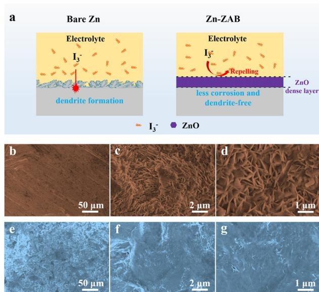
Fig. 4 (a) Schematic diagram of the protective mechanism of the zinc oxide film for bare Zn and Zn-ZAB electrodes for the Zn–I<sub>2</sub> battery. (b–d) SEM images of the bare Zn electrode before (b) and after cycling (c and d). (e–g) SEM images of the Zn-ZAB electrode before (e) and after cycling (f and g).
