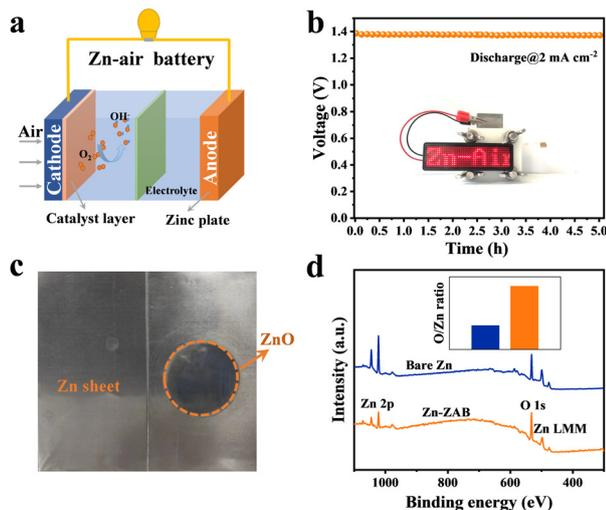
**Fig. 1** (a) Schematic illustration of an as-assembled Zn–air battery. (b) Discharge profile of a Zn–air battery under  $2 \text{ mA cm}^{-2}$ . (c) Photograph of the bare Zn foil and the discharged Zn-ZAB electrode derived from (b). (d) XPS survey of the bare Zn and the Zn-ZAB electrodes (the inset shows the O/Zn ratio of the two electrodes).
