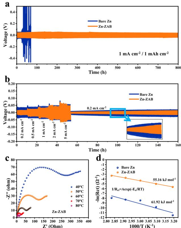
**Fig. 2** (a) Cycling performance of symmetric cells with bare Zn and Zn-ZAB electrodes at a current density of  $1.0 \text{ mA cm}^{-2}$ . (b) Cycling performance of symmetric cells with bare Zn and Zn-ZAB electrodes at different current densities ranging from  $0.2$  to  $5 \text{ mA cm}^{-2}$ . (c) Nyquist plots at different temperatures of the Zn-ZAB electrode symmetric cells. (d) Corresponding Arrhenius curves and the calculated activation energies of bare Zn and Zn-ZAB electrodes.
