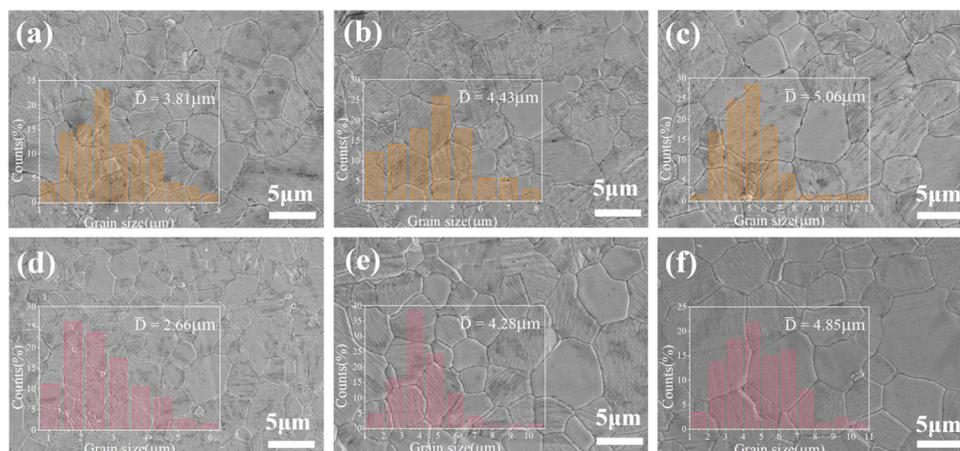
Fig. 3 Polished and thermally etched SEM images of the  $\text{Li}_{10}\text{ZnTi}_{13}\text{O}_{32}$  ceramic sintered at (a) 940  $^\circ\text{C}$ , (b) 980  $^\circ\text{C}$ , and (c) 1020  $^\circ\text{C}$ , and the  $\text{Li}_{10}\text{MgTi}_{13}\text{O}_{32}$  ceramic sintered at (d) 940  $^\circ\text{C}$ , (e) 980  $^\circ\text{C}$ , and (f) 1020  $^\circ\text{C}$ .
