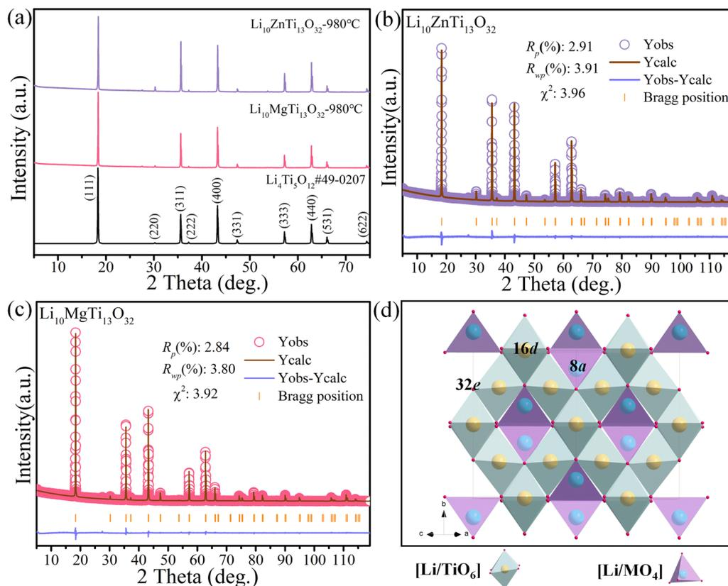
Fig. 1 (a) XRD patterns of the  $\text{Li}_{10}\text{MTi}_{13}\text{O}_{32}$  ( $M = \text{Zn}, \text{Mg}$ ) ceramics sintered at the optimum temperature. Rietveld refinement patterns of (b)  $\text{Li}_{10}\text{ZnTi}_{13}\text{O}_{32}$  and (c)  $\text{Li}_{10}\text{MgTi}_{13}\text{O}_{32}$ . (d) Schematic diagram of the crystal structure of spinel-type  $\text{Li}_{10}\text{MTi}_{13}\text{O}_{32}$  ( $M = \text{Zn}, \text{Mg}$ ).
