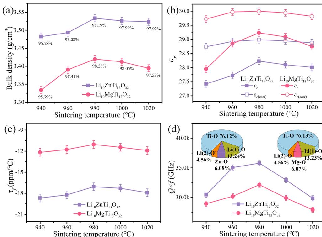
Fig. 4 (a) Density, (b)  $\epsilon_r$ , (c)  $\tau_f$ , and (d)  $Q \times f$  of the  $\text{Li}_{10}\text{MTi}_{13}\text{O}_{32}$  ( $M = \text{Zn, Mg}$ ) samples as a function of the sintering temperature, the inset in (d) shows the contribution of each bond to the lattice energy.
