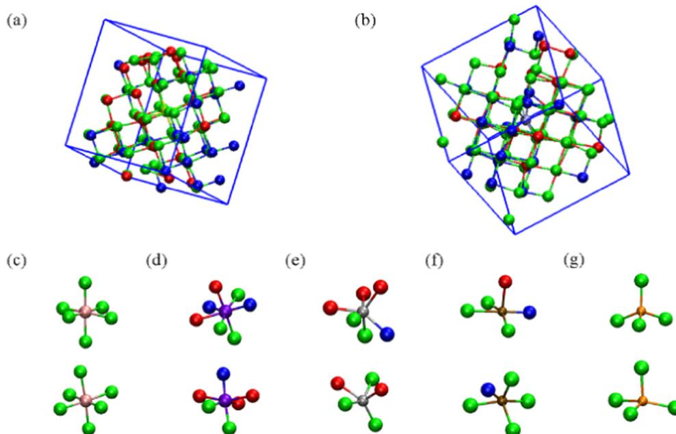
Fig. 9 Structure and bonding in transition-metal (TM)-doped  $\text{Ge}_2\text{Sb}_2\text{Te}_5$ . (a) Sc-, (b) V-, (c) Cr-, (d) Co-, (e) Ni-, (f) Cu-, and (g) Zn-doped GST in amorphous (top) and crystalline (bottom) models. The green, red and blue balls represent Te, Sb, and Ge atoms, respectively. Adapted with permission from ref. 132. ©2006 IOP.
