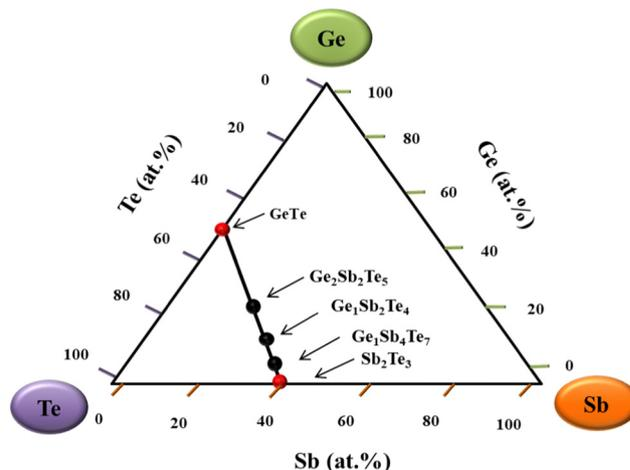
Fig. 2 Pseudo-binary tie line of GeTe and  $Sb_2Te_3$  with ternary compositions ( $Ge_2Sb_2Te_5$ ,  $Ge_1Sb_2Te_4$ , and  $Ge_1Sb_4Te_7$ ) lying between them.<sup>34</sup>
