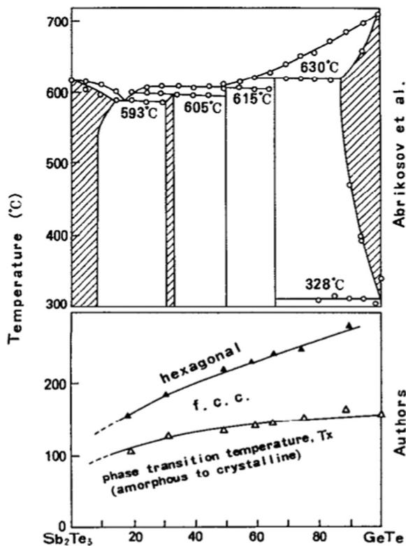
Fig. 4 The pseudo-binary phase diagram of GeTe-Sb<sub>2</sub>Te<sub>3</sub> and the phase transition temperature of various compositions lying on it. Adapted with permission from ref. 34. ©1991 American Institute of Physics.
