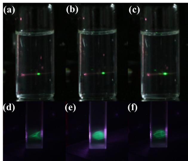
Fig. 9 The TSTF UCL photographs of (a) NaYF<sub>4</sub>:0.5%Er, (b) NaYF<sub>4</sub>:0.5%Er@NaGdF<sub>4</sub>:2%Yb and (c) NaYF<sub>4</sub>:0.5%Er@NaGdF<sub>4</sub>:2%Yb@NaYF<sub>4</sub>:1%Er UCNPs. 3-D image of (d) triangular pyramid, (e) sphere and (f) hollow dodecahedron of NaYF<sub>4</sub>:0.5%Er@NaGdF<sub>4</sub>:2%Yb@NaYF<sub>4</sub>:1%Er UCNPs under 850 & 1550 nm excitation.
