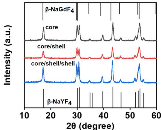
Fig. 3 XRD patterns of NaYF $_4$ :0.5%Er, NaYF $_4$ :0.5%Er@NaGdF $_4$ :2%Yb, NaYF $_4$ :0.5%Er@NaGdF $_4$ :2%Yb@NaYF $_4$ :1%Er UCNPs and standard date of  $\beta$ -NaYF $_4$  (JCPDS No. 16-0334) and  $\beta$ -NaGdF $_4$  (JCPDS No. 27-0699).
