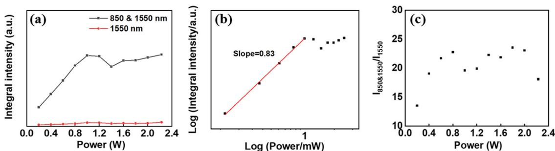
Fig. 7 (a and b) The pump power dependence of UCL integral intensities of  $\text{NaYF}_4:0.5\%\text{Er}@NaGdF_4:2\%\text{Yb}@NaYF_4:1\%\text{Er}$  UCNPs on 1550 nm laser power. (c) The pump power dependence of UCL contrast on 1550 nm laser power. The 850 nm laser power is maintained at 0.2 W.
