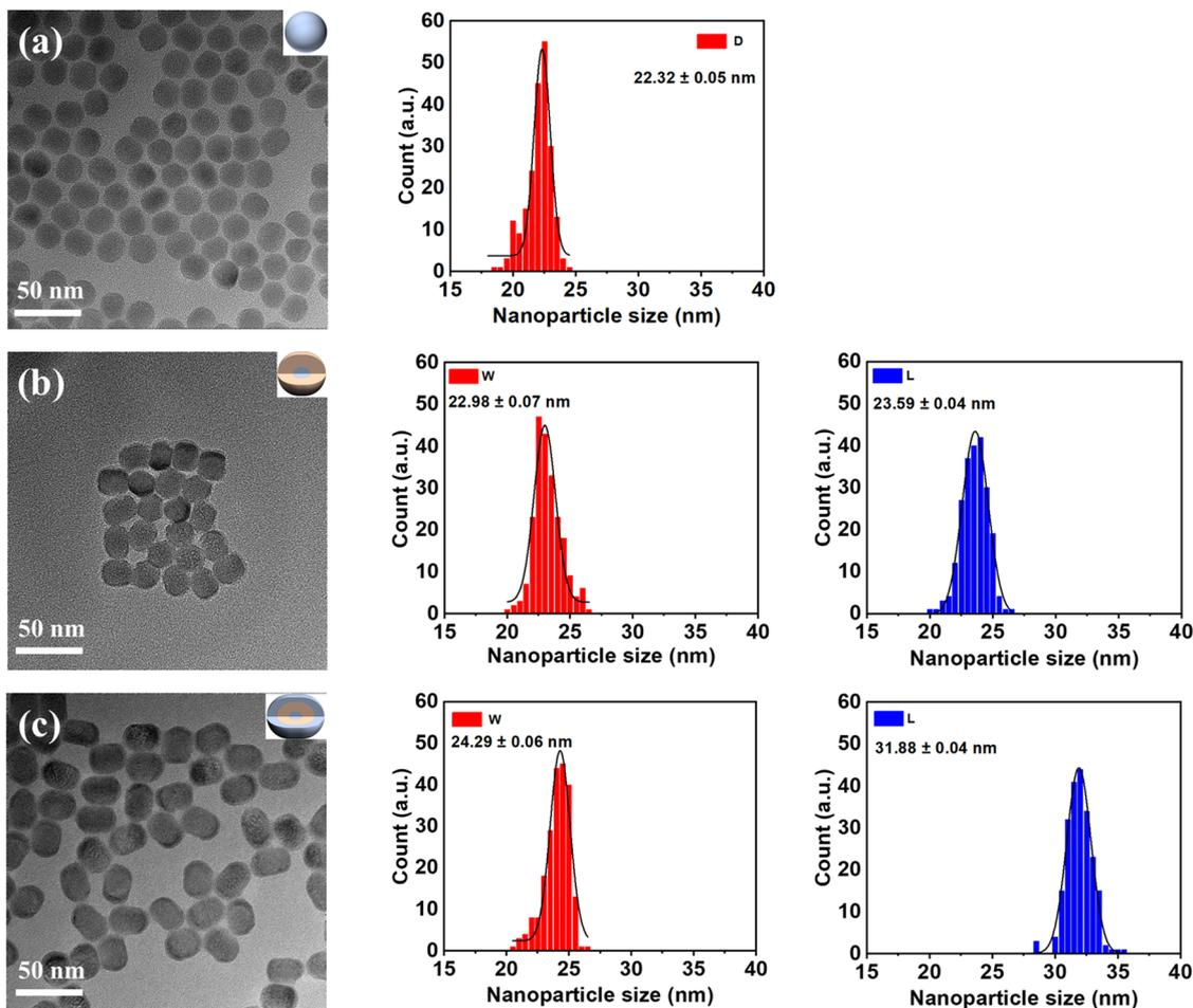
Fig. 4 TEM images of UCNPs (left) and the corresponding size distributions of UCNPs (right). (a)  $\text{NaYF}_4:0.5\%\text{Er}$ , (b)  $\text{NaYF}_4:0.5\%\text{Er}@NaGdF_4:2\%\text{Yb}$ , and (c)  $\text{NaYF}_4:0.5\%\text{Er}@NaGdF_4:2\%\text{Yb}@NaYF_4:1\%\text{Er}$  UCNPs. The size distributions of the UCNPs were calculated by counting over 200 particles recorded in the TEM images.
