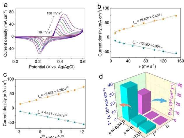
**Fig. 3** (a) CV curves of the a-Ni-Bi/Ni<sub>x</sub>B hybrid measured in 1 M KOH solution at different scan rates (10, 20, 50, 75, 100, 120 and 150 mV s<sup>-1</sup>). The corresponding linear relationships between the anodic and cathodic current densities and (b) the scan rates, and (c) the square root of the scan rates. (d) The calculated  $\Gamma^*$  values and  $D$  values for the a-Ni-Bi/Ni<sub>x</sub>B hybrid, a-Ni<sub>x</sub>B and a-Ni-Bi samples.
