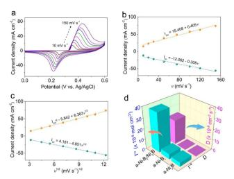
Fig. 3 (a) CV curves of the a-Ni-B<sub>i</sub>/Ni<sub>x</sub>B hybrid measured in 1 M KOH solution at different scan rates (10, 20, 50, 75, 100, 120 and 150 mV s<sup>-1</sup>). The corresponding linear relationships between the anodic and cathodic current densities and (b) the scan rates, and (c) the square root of the scan rates. (d) The calculated  $\Gamma$ \* values and D values for the a-Ni-B<sub>i</sub>/Ni<sub>x</sub>B hybrid, a-Ni<sub>x</sub>B and a-Ni-B<sub>i</sub> samples.
