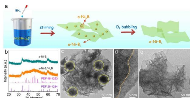
Fig. 1 (a) Schematic diagram for the fabrication of  $\text{a-Ni-B}_i/\text{Ni}_x\text{B}$  hybrid and  $\text{a-Ni-B}_i$  nanosheets. (b) XRD patterns of the as-prepared  $\text{a-Ni-B}_i/\text{Ni}_x\text{B}$  hybrid and  $\text{a-Ni-B}_i$  samples. (c) TEM and (d) HRTEM images of the  $\text{a-Ni-B}_i/\text{Ni}_x\text{B}$  hybrid sample. (e) TEM image of the ultrathin  $\text{a-Ni-B}_i$  nanosheets.
