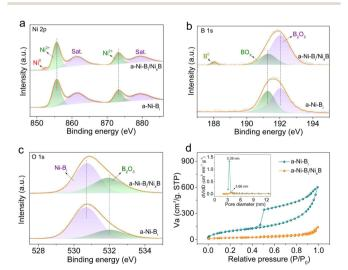
Fig. 2 High-resolution XPS spectra of (a) Ni 2p, (b) B 1s, and (c) O 1s, and (d) nitrogen adsorption-desorption isotherms and the corresponding pore size distribution curves (inset) of the a-Ni-B<sub>i</sub>/Ni<sub>x</sub>B hybrid and a-Ni-B<sub>i</sub> samples
