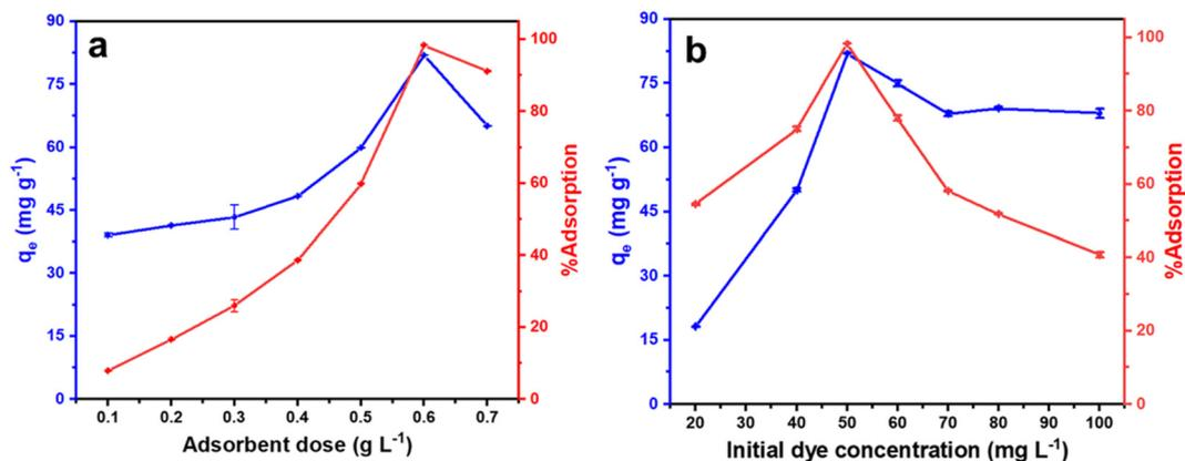
Fig. 6 Effect of (a) adsorbent dose at a fixed dye concentration of 50 mg L<sup>-1</sup> and (b) initial dye concentration at a fixed adsorbent dose of 0.6 g L<sup>-1</sup> on the adsorption performance of CeO<sub>2</sub> NPs (sample CeO-2). Condition: temperature (303 K); pH (~7).
