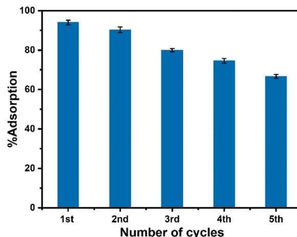
**Fig. 9** Performance of the used CeO<sub>2</sub> NPs in malachite green dye removal.
