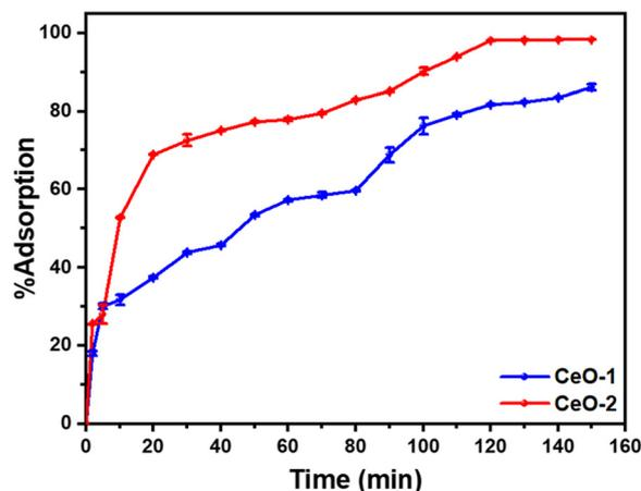
Fig. 5 Variation of %adsorption of malachite green dye with time on different samples of CeO<sub>2</sub> NPs. Conditions: initial malachite green dye concentration (50 mg L<sup>-1</sup>); adsorbent dose (0.6 g L<sup>-1</sup>); time (150 min); temperature (303 K); pH (~7).
