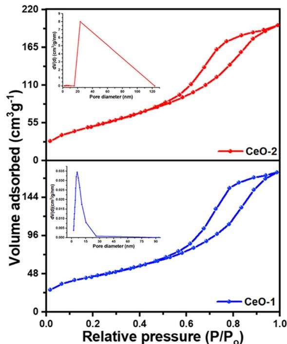
Fig. 3 N<sub>2</sub> gas adsorption–desorption isotherms of different samples of CeO<sub>2</sub> NPs. Insets in the figure represent the BJH plots of the pore size distribution of the respective samples.
