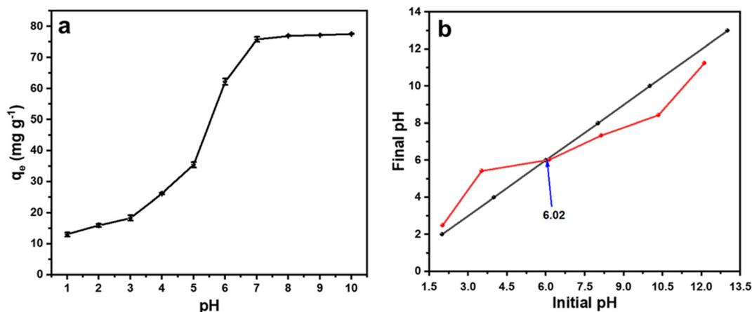
Fig. 7 (a) The effect of pH on the adsorption performance of CeO<sub>2</sub> NPs (sample CeO-2) and (b) plot of final pH versus initial pH obtained using the pH drift method.
