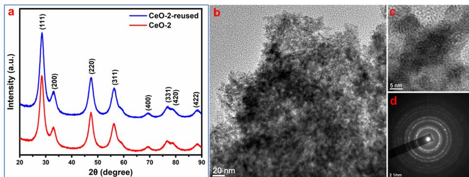
Fig. 10 (a) XRD pattern and (b) TEM image of recovered CeO<sub>2</sub> NPs. (c) HRTEM image and (d) SAED pattern of the respective sample.
