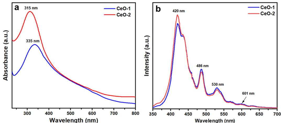
Fig. 4 (a) UV-vis absorption spectra and (b) room temperature PL spectra of different samples of CeO<sub>2</sub> NPs. The PL spectra were recorded at an excitation wavelength of 320 nm.
