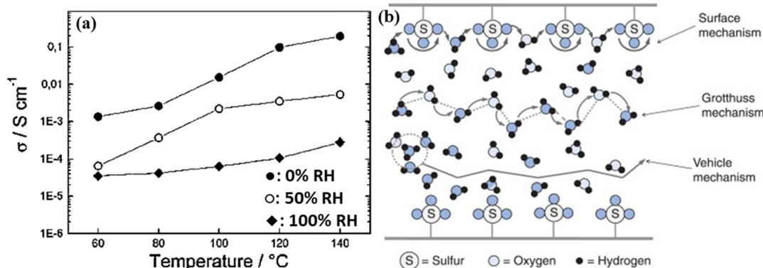
Fig. 16 (a) Proton conductivity of 40% SO<sub>3</sub>H-MCM-41 (mw) at 0% (◆), 50% (○), and 100% (●) RH, Reprinted with permission from *Chem. Mater.* **19**, 26 (2007): 6401–6407. Copyright (2007) American Chemical Society.<sup>74</sup> and (b) simplified schematic representation of proton transport via the surface mechanism, Grotthuss mechanism, and vehicle mechanism.<sup>75</sup>
