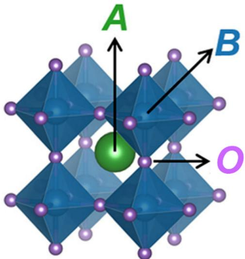
Fig. 1 The ideal structure of  $ABO_3$ .<sup>13</sup>
