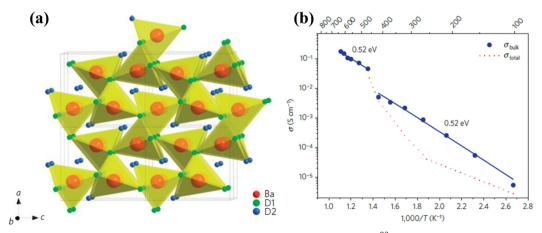
Fig. 18 (a) Crystal structure of  $BaD_2$ , and (b) Arrhenius plot of hydride-anion conductivity of  $BaH_2$ .
