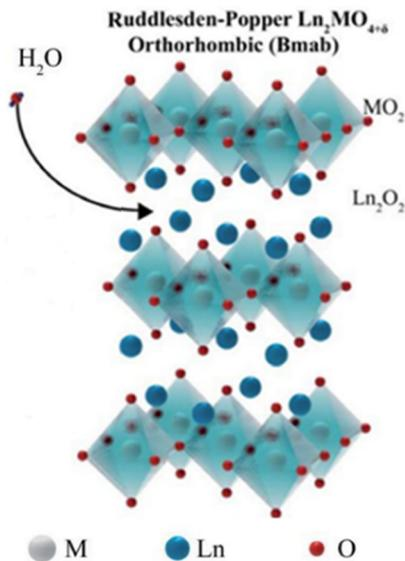
Fig. 7 The crystal structure of  $\text{Ln}_2\text{MO}_{4+\delta}$  with the arrow indicating the possible water insertion sites.<sup>36</sup>
