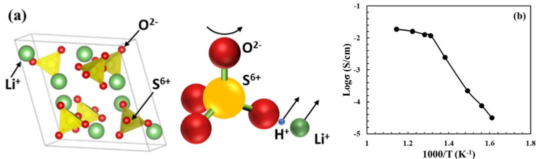
Fig. 10 (a) Crystal structure of the face-centered cubic  $\alpha$ - $\text{Li}_2\text{SO}_4$ , where  $\text{SO}_4$  tetrahedron and its rotation pushing out of  $\text{Li}^+$  and  $\text{H}^+$  are illustrated.<sup>49</sup> (b) Arrhenius plot of proton conductivity of  $\text{Li}_2\text{SO}_4$ -45 mol% $\text{Al}_2\text{O}_3$  (reproduced from ref. 50).
