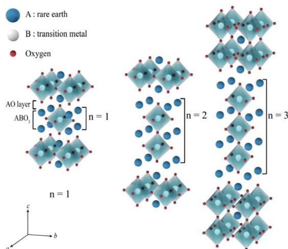
Fig. 6 Idealized representation of the crystal structures of Ruddlesden-Popper (RP) phases.<sup>36</sup>
