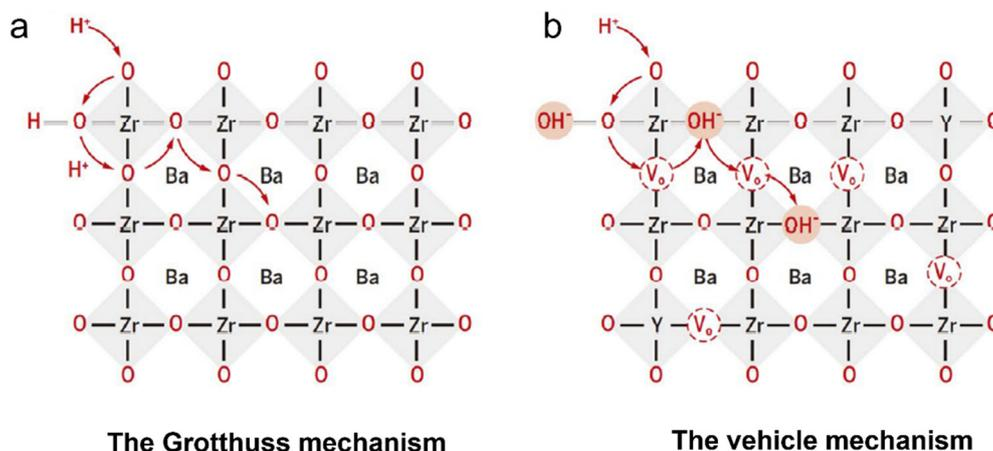
Fig. 2 Schematics of two  $\text{H}^+$  conducting mechanisms in a  $\text{BaZrO}_3$ -based perovskite oxide: (a) the Grotthuss mechanism and (b) the vehicle mechanism.<sup>17</sup>
