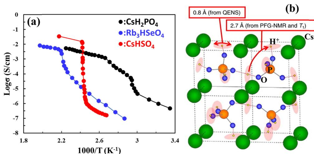
Fig. 14 (a) Arrhenius plot of proton conductivity of  $\text{CsH}_2\text{PO}_4$ ,  $\text{Rb}_3\text{HSeO}_4$ , and  $\text{CsHSO}_4$  (reproduced from ref. 55) and (b) illustration of two proton diffusion movements in  $\text{CsH}_2\text{PO}_4$ , confirmed via  $^1\text{H}$  pulsed field gradient NMR,  $^1\text{H}$  NMR spin-lattice relaxation time ( $T_1$ ), and quasi-elastic neutron scattering measurements.<sup>70</sup>
