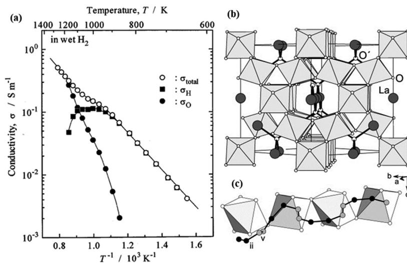
Fig. 8 (a) Arrhenius plot of conductivity of  $(\text{La}_{1.95}\text{Ca}_{0.05})\text{Zr}_2\text{O}_7$  in wet  $\text{H}_2$ , (■)  $\sigma_{\text{H}}$ , (●)  $\sigma_{\text{O}}$  and (○)  $\sigma_{\text{total}}$  represent partial proton, oxide-ion conductivity, and total conductivity, respectively;<sup>43</sup> (b)  $\text{La}_2\text{Zr}_2\text{O}_7$  structure; (c) suggested proton conduction pathway.<sup>44</sup>
