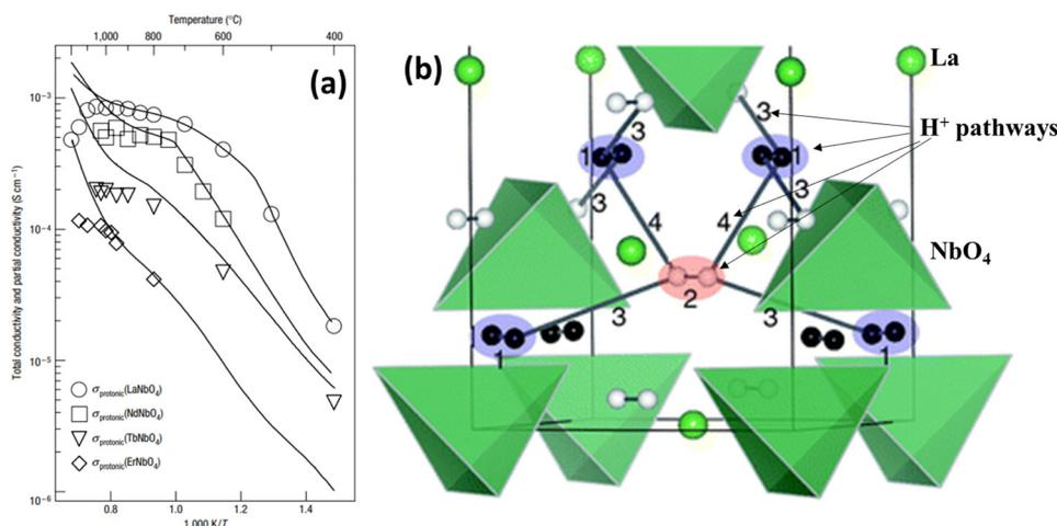
Fig. 9 (a) Protonic conductivities of 1% Ca-doped RENbO<sub>4</sub>,<sup>45</sup> (b) proton migration paths with low potential barriers in the tetragonal phase of LaNbO<sub>4</sub>. Proton migration pathways are labelled as 1–4 in the figure.<sup>47</sup>
