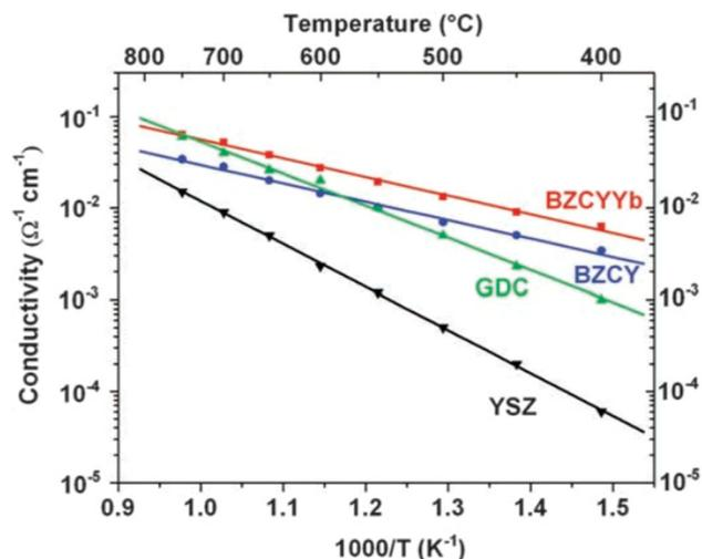
Fig. 3 Ionic conductivities of BZCYYb, BZCY, GDC, and YSZ as measured at 400° to 750 °C in wet oxygen (with ~3 vol % H<sub>2</sub>O).<sup>23</sup>
