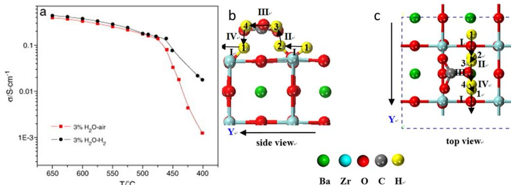
Fig. 5 Plots of effective ionic conductivity of BZY-(Li<sub>0.62</sub>K<sub>0.38</sub>)<sub>2</sub>CO<sub>3</sub> (MC) (a) vs. temperature in 3% H<sub>2</sub>O-air and 3% H<sub>2</sub>O-H<sub>2</sub>.<sup>32</sup> Migration pathways for H<sup>+</sup> migration along the Y direction in MPCC, (b) side view and (c) top view. The migration pathways are marked with arrows.<sup>33</sup>
