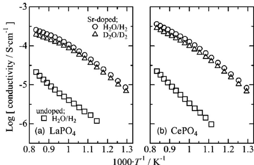
Fig. 12 Conductivities of undoped and 1 mol % Sr-doped (a)  $\text{LaPO}_4$  and (b)  $\text{CePO}_4$  under wet reducing conditions;  $p_{\text{H}_2\text{O}}$  or  $p_{\text{D}_2\text{O}} = 4.2$  kPa, and  $p_{\text{H}_2}$  or  $p_{\text{D}_2} = 3$  kPa.<sup>56</sup>
