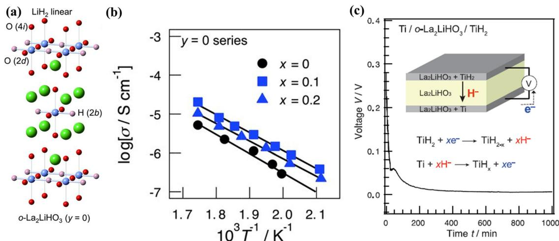
Fig. 19 (a) The crystal structure of  $o$ - $\text{La}_2\text{LiH}_3\text{O}_3$ , (b) Arrhenius plot of the ionic conductivity of  $\text{La}_{2-x}\text{Sr}_x\text{LiH}_{1-x}\text{O}_3$  ( $y = 0, 0 \leq x \leq 0.2$ ), and (c) discharge curve of cell  $\text{Ti}/o\text{-La}_2\text{LiHO}_3/\text{TiH}_2$ . The inset shows the cell configuration and the proposed electrochemical reactions.<sup>95</sup>
