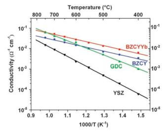
Fig. 3 Ionic conductivities of BZCYYb, BZCY, GDC, and YSZ as measured at 400° to 750 °C in wet oxygen (with  $\sim$  3 vol % H<sub>2</sub>O).<sup>23</sup>
