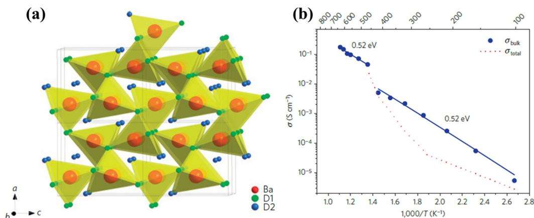
Fig. 18 (a) Crystal structure of  $\text{BaD}_2$ , and (b) Arrhenius plot of hydride-anion conductivity of  $\text{BaH}_2$ .<sup>92</sup>
