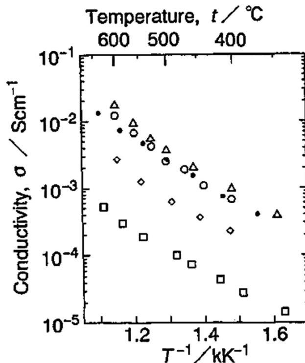
Fig. 22 Arrhenius plots of conductivity of LiBaF<sub>3-x</sub>H<sub>x</sub> in H<sub>2</sub>: □  $x = 0$ , ◇  $x = 0.05$ , ○  $x = 0.1$ , △  $x = 0.2$ , ● LiBa<sub>0.9</sub>K<sub>0.1</sub>F<sub>2.8</sub>H<sub>0.1</sub>.<sup>106</sup>
