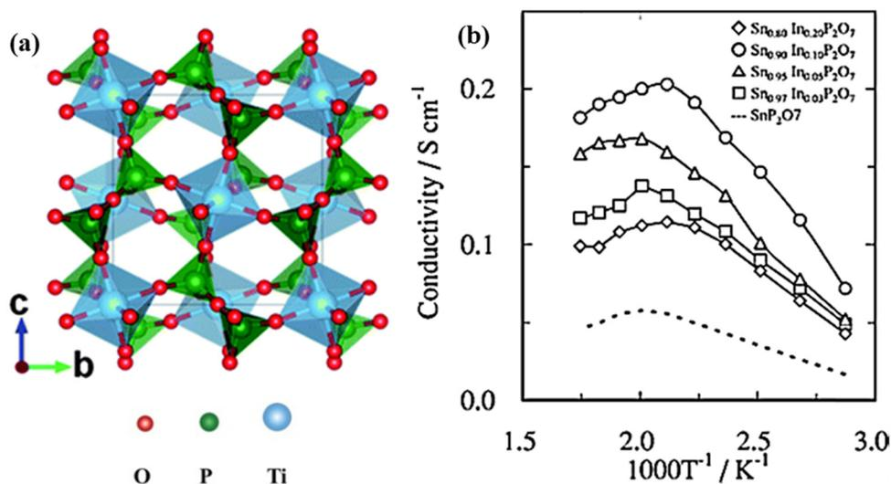
Fig. 13 (a) Crystal structure of  $\text{TiP}_2\text{O}_7$ ,<sup>66</sup>  $\text{TiO}_6$  octahedra and  $\text{PO}_4$  tetrahedra are shown in blue and green in color, respectively, and (b) Arrhenius plot of the conductivity of  $\text{Sn}_{1-x}\text{In}_x\text{P}_2\text{O}_7$  in dry air ( $p_{\text{H}_2\text{O}} = \sim 0.0075$  atm).<sup>65</sup>
