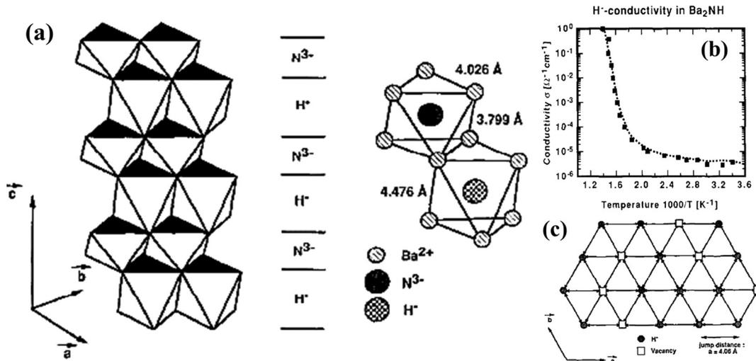
Fig. 21 (a) Layered type structure of Ba<sub>2</sub>NH with distorted Ba-octahedra centered alternately by H<sup>-</sup> and N<sup>3-</sup>, with corresponding distance, (b) Arrhenius plot of H<sup>-</sup> conductivity in Ba<sub>2</sub>NH, and (c) diffusion of hydride anions in Ba<sub>2</sub>NH via uncorrelated jumps between regular hydrogen sites.<sup>101</sup>
