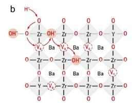
The vehicle mechanism
