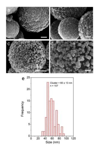
**Fig. 3** SEM micrographs of precursor and composite systems prepared using approach 2: (a) **CA-CμP**, (b) **CμP-AuNP(BH)** and (c and d) roughened composites **CμP-AuNP-2**. Scale bars show (a and b) 100 nm; (c) 500 nm; and (d) 50 nm.
