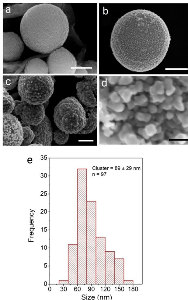
Fig. 1 SEM micrographs of precursor and composite systems prepared using approach 1: (a) **o- $C_{\mu}P$** , (b)  **$C_{\mu}P$ -AuNP(DMAP)** and (c and d) and roughened composites  **$C_{\mu}P$ -AuNP-1**. Scale bars show (a–c) 500 nm and (d) 50 nm.
