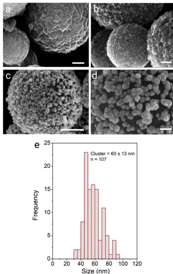
Fig. 3 SEM micrographs of precursor and composite systems prepared using approach 2: (a) CA-C $\mu$ P, (b) C $\mu$ P-AuNP(BH) and (c and d) roughened composites C $\mu$ P-AuNP-2. Scale bars show (a and b) 100 nm; (c) 500 nm; and (d) 50 nm.
