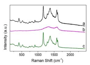
Fig. 5 Raman spectrum of: (a) individual trapped  $C\mu P$ -AuNP-1 incubated with 10  $\mu M$  of MG (black trace); (b) reference spectrum from averaged CμP-AuNP-1 particle spectra in the absence of MG; (c) MG-incubated CμP-AuNP-1 particle following subtraction of reference spectrum. All spectra recorded in H<sub>2</sub>O with 785 nm excitation.
