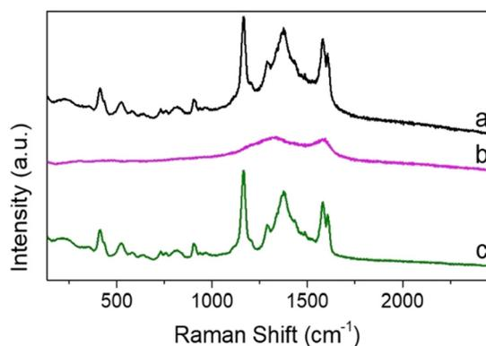
Fig. 5 Raman spectrum of: (a) individual trapped **C $\mu$ P-AuNP-1** incubated with 10  $\mu$ M of **MG** (black trace); (b) reference spectrum from averaged **C $\mu$ P-AuNP-1** particle spectra in the absence of **MG**; (c) **MG**-incubated **C $\mu$ P-AuNP-1** particle following subtraction of reference spectrum. All spectra recorded in H<sub>2</sub>O with 785 nm excitation.
