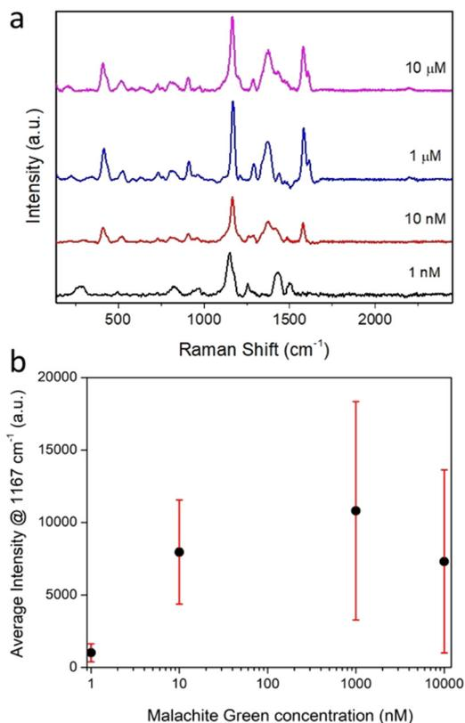
**Fig. 6** (a) SERS spectra for **C $\mu$ P-AuNP-1** composite particles incubated with **MG** at concentrations of 1 nM to 10  $\mu$ M. Spectra shown are from the highest intensity measurement from each MG concentration. Each trace shows an individual particle. (b) Average SERS intensity for the 1167  $\text{cm}^{-1}$  peak as a function of **MG** incubation concentration. Spectra recorded in  $\text{H}_2\text{O}$  with 785 nm excitation.
