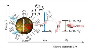
Fig. 18 Singlet oxygen generation production via energy transfer from dye-functionalized SiQDs to Oxygen. Reproduced with permission from ref. 54. Copyright (2020) Frontier in Chemistry.
