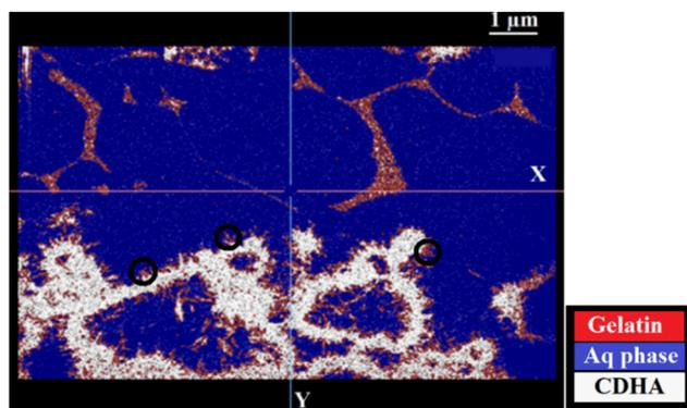
**Fig. 2** Segmentation of the different phases in a BSE image of a CDHA/gelatin compound using the random forest trainer method incorporated in the Dragonfly<sup>®</sup> software.<sup>39</sup>
