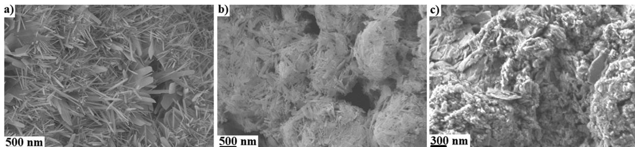
Fig. 7 (a) SEM micrographs of (a) CDHA (b) CDHA mixed with gelatin<sup>52</sup> and (c) CDHA mixed with Si-HA.
