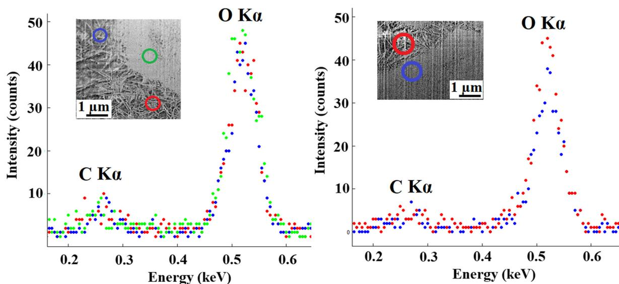
Fig. 6 Comparison between EDS spectra acquired at different regions in two randomly selected CDHA/Si-HA particles. EDS measurements were performed using electron energies of 1.7 keV for the first particle (left hand side) and 2 keV for the second particle (right hand side).
