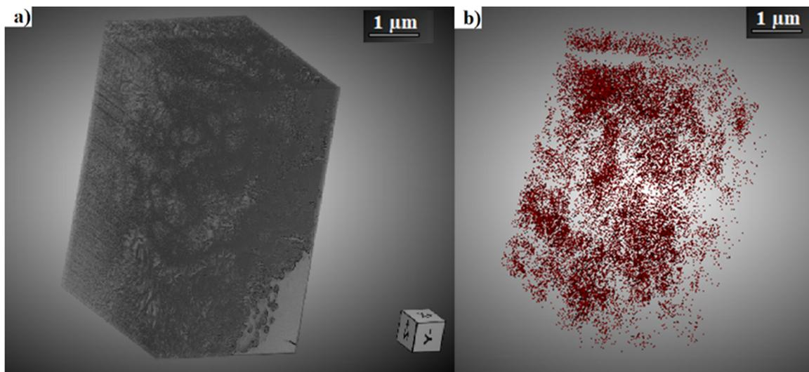
Fig. 9 (a) 3D reconstruction of the anhydrous CDHA sample using the Dragonfly<sup>®</sup> software.<sup>39</sup> (b) 3D pore mesh inside the reconstructed volume.
