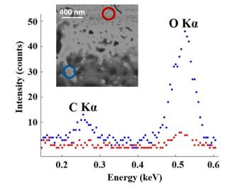
Fig. 3 Comparison between EDS spectra acquired at different regions in two randomly selected CDHA/gelatin particles. EDS spectra were acquired using an electron energy of 1.6 keV.
