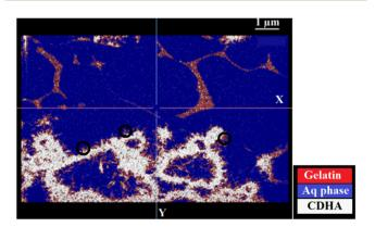
Fig. 2 Segmentation of the different phases in a BSE image of a CDHA/ gelatin compound using the random forest trainer method incorporated in the Dragonfly  $^{\text{(E)}}$  software.  $^{39}$
