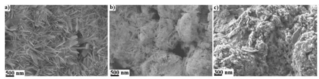
Fig. 7 (a) SEM micrographs of (a) CDHA (b) CDHA mixed with gelatin<sup>52</sup> and (c) CDHA mixed with Si-HA
