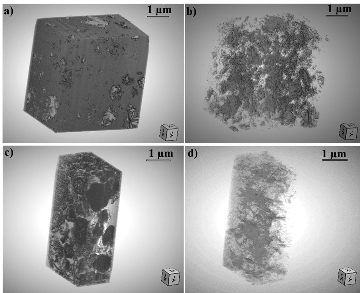
Fig. 10 (a) 3D reconstructed volume of the anhydrous CDH/gelatin sample using the Dragonfly<sup>®</sup> software.<sup>39</sup> (b) 3D pore mesh inside the CDHA/gelatin reconstructed volume. (c) 3D volume of anhydrous CDH/Si-HA and its (d) 3D corresponding pores mesh.
